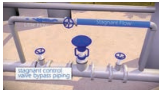
Figure 1. Dead leg example: control valve bypass.
