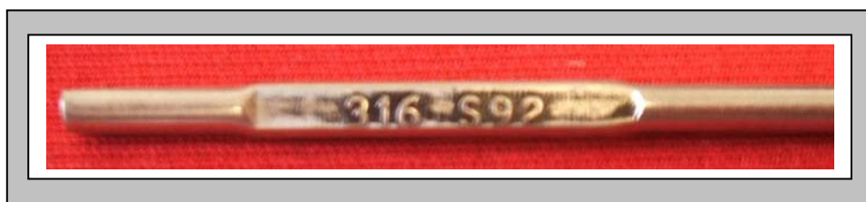
TIG consumable identification is stamped at the end of the wire
