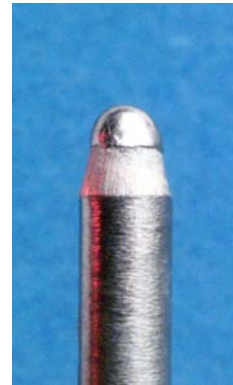
electrode tip with a 'balled' end
