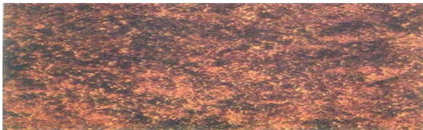
Rust Grade C Steel surface on which the mill scale has rusted away or from which it can be scrapped. Slight pitting visible under normal vision.
