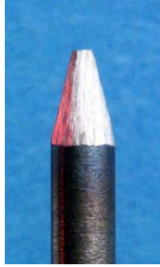
electrode tip with flat end
