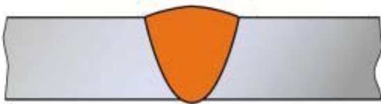
Single run weld
