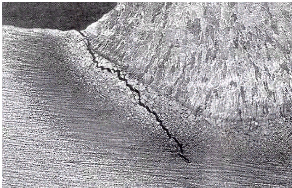
Figure 2 A hydrogen induced cold crack that initiated the HAZ at the toe of a fillet weld
