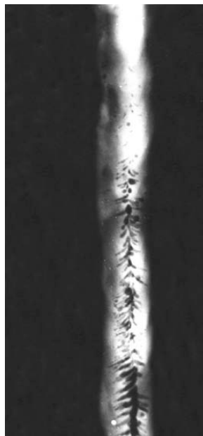
Figure 3: X-Ray of a welded seam showing Porosity
