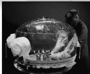
Welding in protective tent
