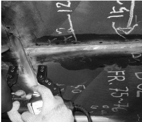
Magnetic particle inspection using a yoke.
