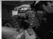
Electro-magnet (yoke) DC or AC
