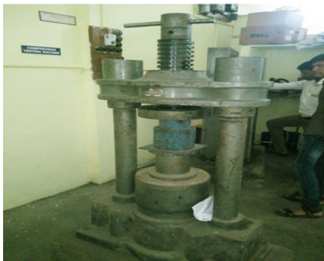
Fig. 3 Crushing value test apparatus (Testing at Concrete Technology Lab. NHCE Parli V.)
