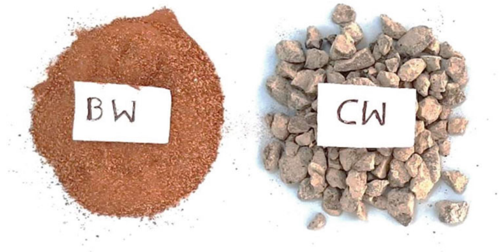
Fig. 2 Demolished BW and CW processed materials
