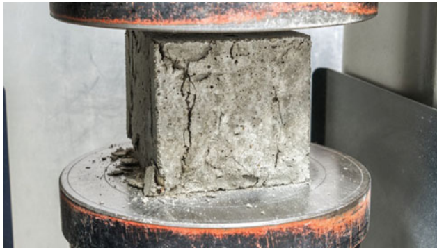
Fig. 5 Compressive test on concrete ( https://www.forconstructionpros.com/ )
