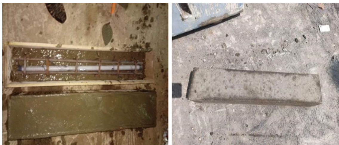
Fig. 1 PVC pipe encased inside concrete beam and casting of the specimen
