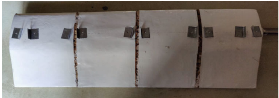
Fig. 5 Fabrication of NRELS809 airfoil with vortex generator and pressure port
