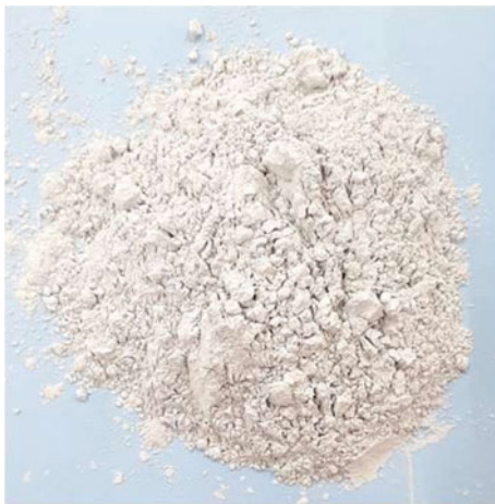
Fig. 3 GGBS by-product from steel manufacturing
