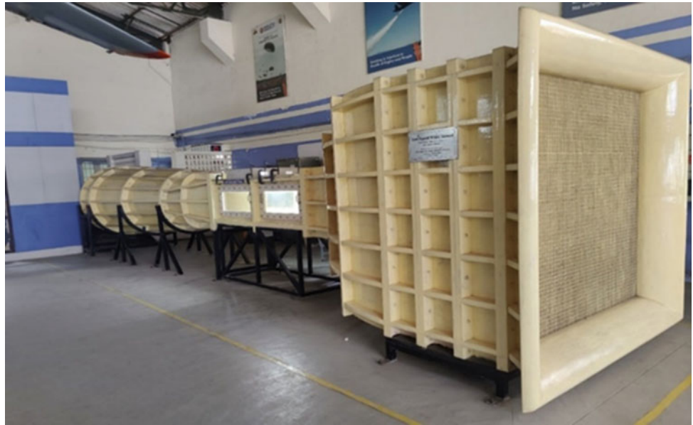
Fig. 2 Low-speed subsonic wind tunnel facility
