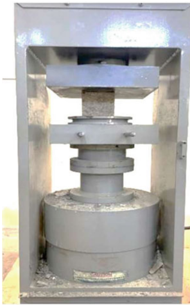
Fig. 5 Compressive strength test of GPC cube under testing equipment
