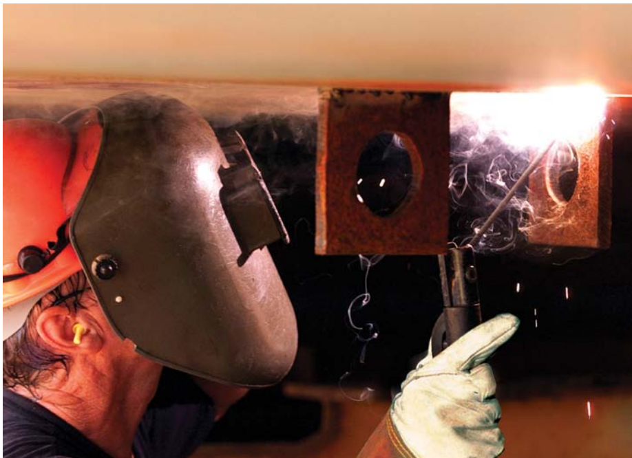
Illustration 5-4 – Shielded Metal Arc Welding used in Ship Construction
