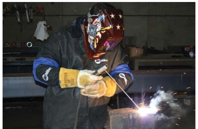
Illustration 5-6 – Shielded Metal Arc Welding in a Shop Setting
