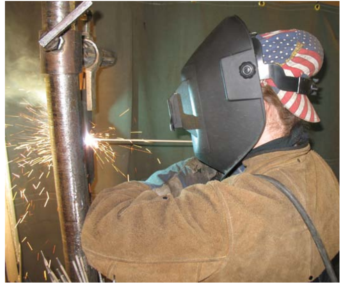
Illustration 14-1 – Basic Shielded Metal Arc Welding
