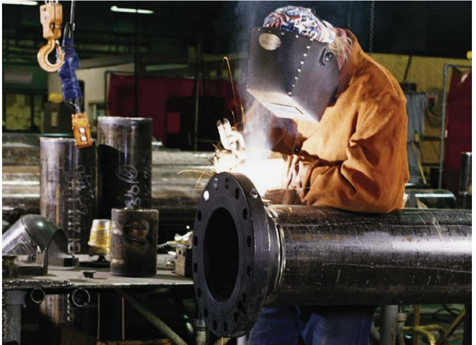
Illustration 5-2 – E7018 Electrode being used to Weld the Cover Pass on a Joint in Industrial Piping
