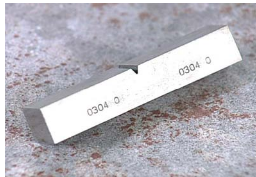
Illustration 7-3 – Charpy V-Notch Bar
