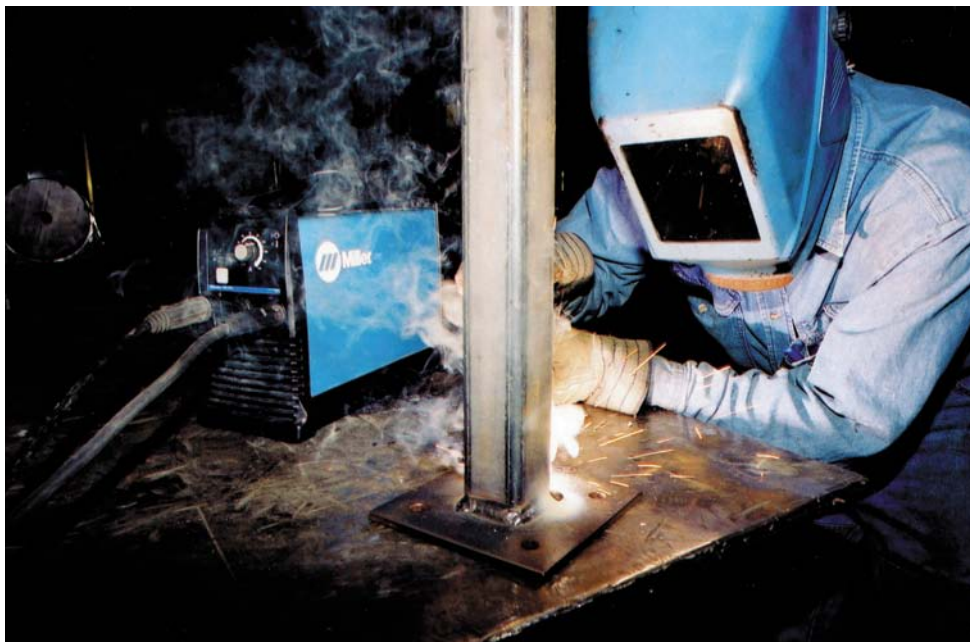
Illustration 5-3 – Welding the Base of a Support Column with the Shielded Metal Arc Welding Process
