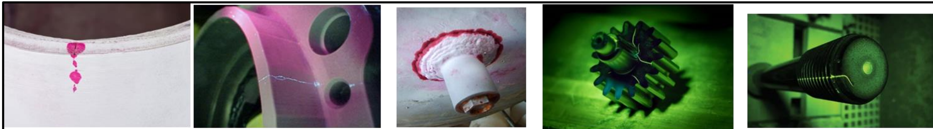
Different types of defects detected by dye penetrant testing
