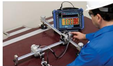
Testing of Composite Structure for Laminar Flaws
