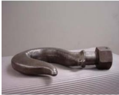
Crane Hook with Service Induced Crack
