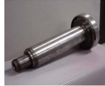
Drive Shaft with Heat Treatment Induced Cracks
