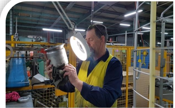
Direct visual inspection of welded parts
