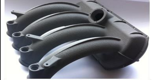
Inlet manifold (polyamide composite reinforced by Al-Cu-Fe-B quasicrystals)
