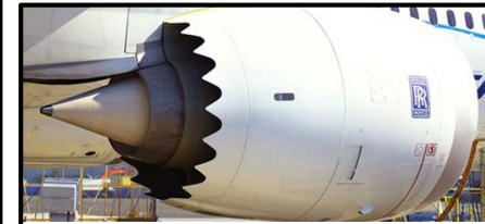
Engine nozzle made from CMCs
