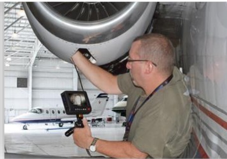
Inspection of Aircraft using Fiberscope
