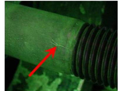
Large Bolt with Service Induced Crack
