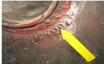
Crack in Seal Weld of Boiler Tube to Steam Drum
