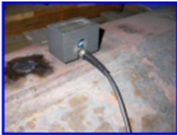
AE Sensor attached with magnet
