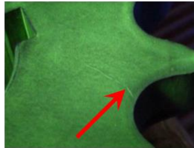
Gear with Service Induced Crack
