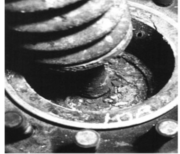
Figure 33—Moving Parts of Valve Fouled with Iron Sulfide ( \text{FeS}_2 )
