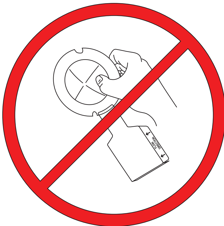
Figure A.3—Improper Handling of a Rupture Disk
