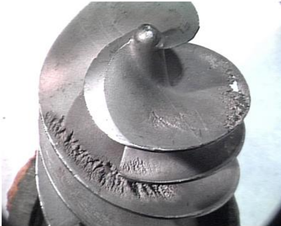
Figure 4-48 – Cavitation pitting on the low-pressure side of a stainless steel pump impeller.
