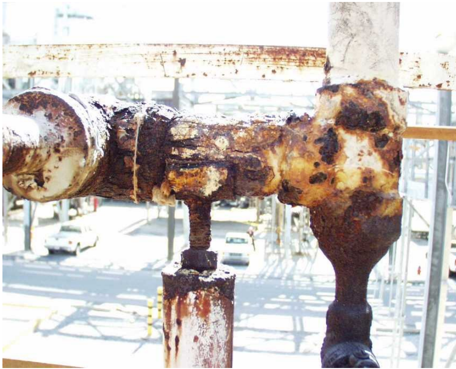
Figure 4-80 – CUI of CS level bridge.
