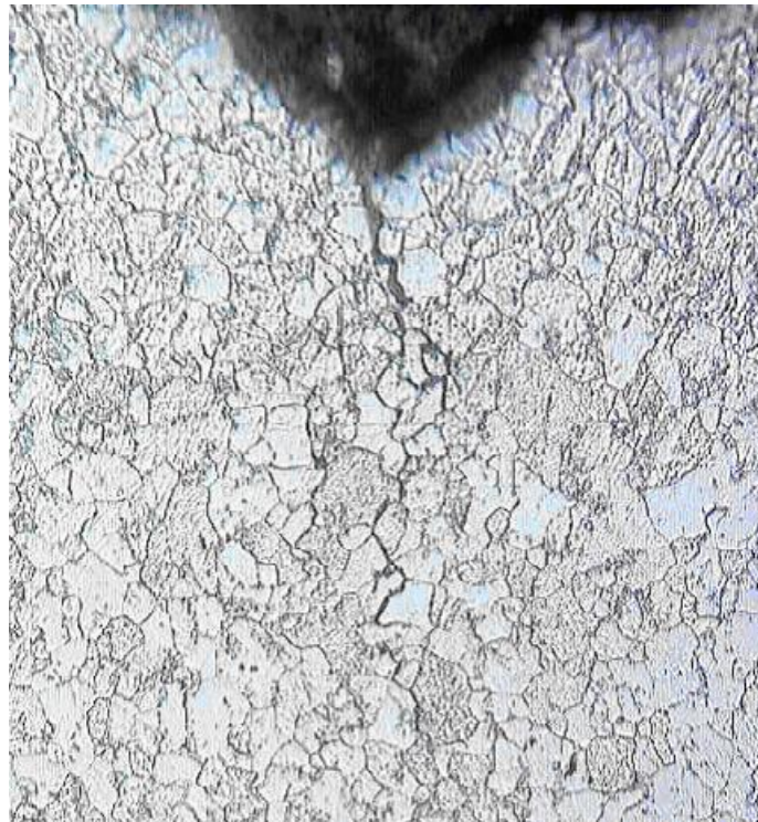
Figure 4-148 – Photomicrograph of a crack in the tube shown in Figure 4-147.
