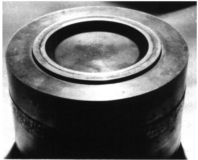
Figure 27—Seating Surface of Disk Deformed by Chattering
