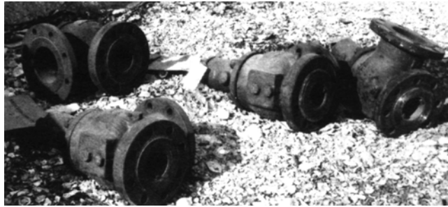
Figure 36—Rough Handling of Valves Should be Avoided
