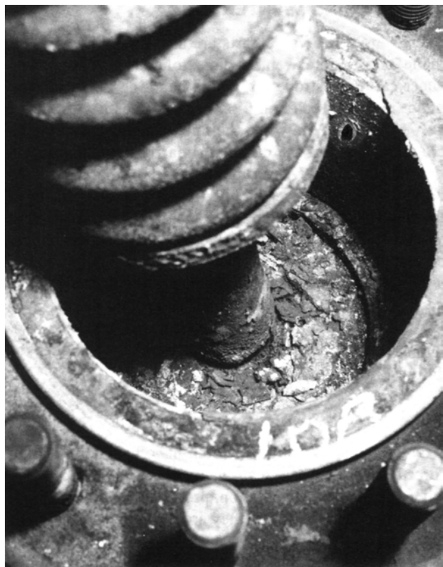
Figure 33—Moving Parts of Valve Fouled with Iron Sulfide ( \text{FeS}_2 )
