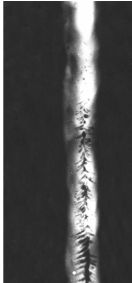
X-ray of a welded seam showing porosity.
