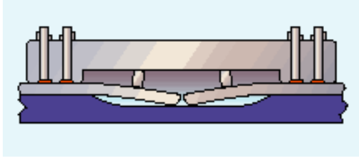
Figure 3 Pre-bending, using strongbacks and wedges, to accommodate angular distortion in thin plates.
