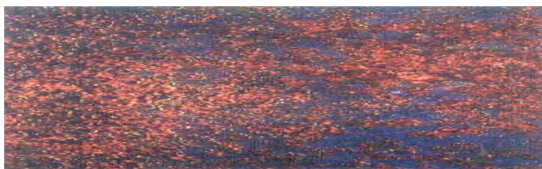
Rust Grade B: Steel surface, which has begun to rust, and from which mill scale has begun to flake.
