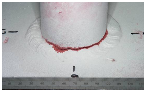
Crack found using dye penetrant inspection.
