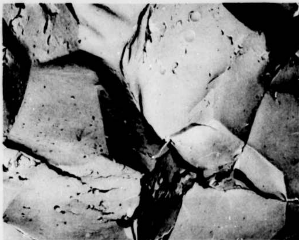
FIGURE 59 Electron Micrograph of Quench Crack Fracture Face. 4340 Water Quenched from 1575°F 4200X
