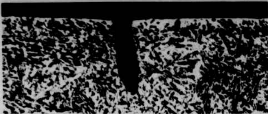
FIGURE 25 Electropolished Surface (with inclusion) Nital 750X
