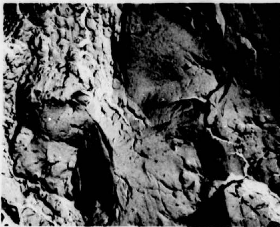
FIGURE 55 Electron Micrograph of Hydrogen Embrittlement Failure 4340 269,000 - 280,000 psi Heat Treat Strength Range 4600X
