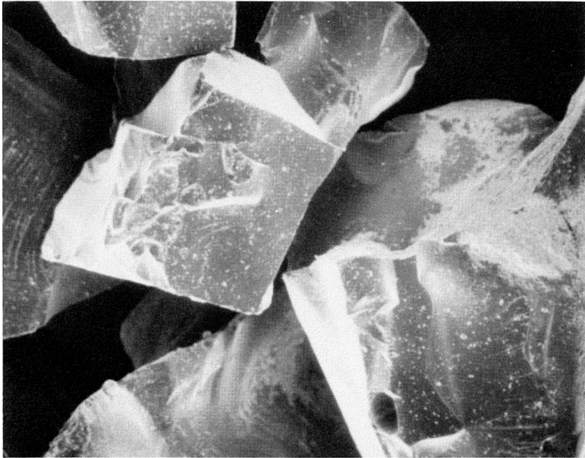
FIGURE 1.23. The appearance of the grains in a fused flux. (Scanning electron micrograph, with gold evaporated on the grain surfaces.)
