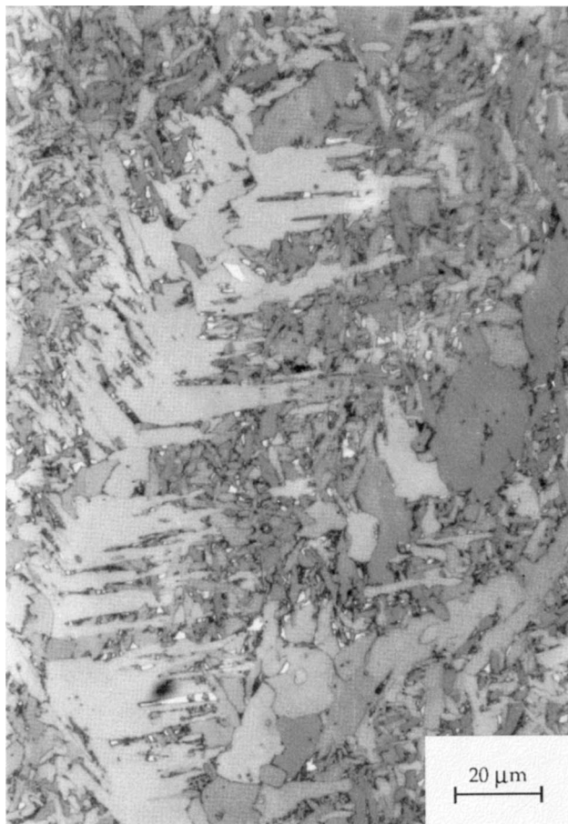
FIGURE 3.3. Widmanstätten side plates, nucleating on ferrite/austenite boundaries (secondary side plates).
