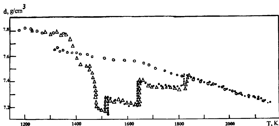
Figure 1.30 Temperature dependences of the density of Ni–22.5 at. % B alloy [185] (• first heating, ◦ cooling, △ repeated heating after solidification).
