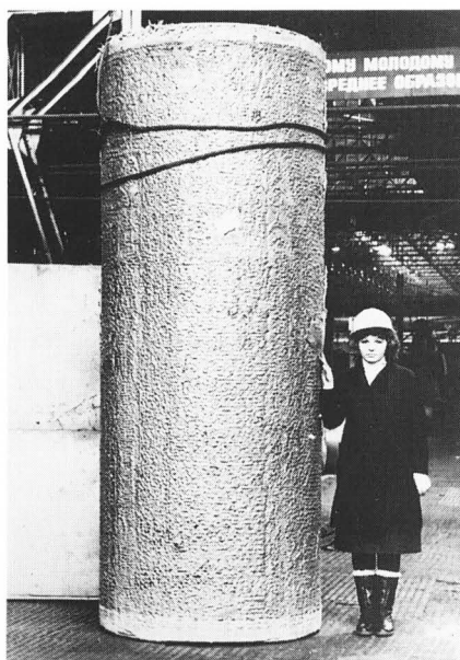
Figure 4.21 One of the largest ingots (1200 mm diameter, 10 ton weight) of alloy 1161 (2324) with non-dendritic structure obtained by casting with UST.
