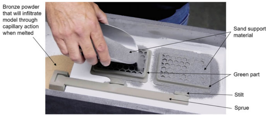
Fig. 10.1 The metal binder jetting bronze infiltration process. Courtesy of ExOne
