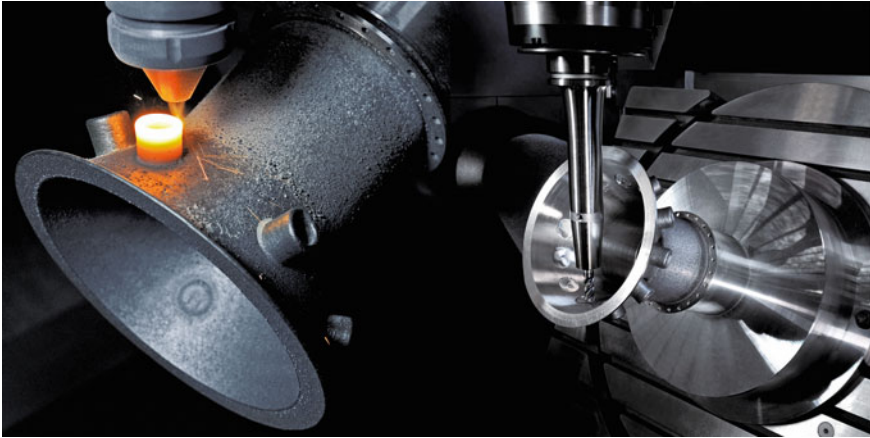
Fig. 2.13 Hybrid directed energy deposition CNC additive manufacturing system. Courtesy of DMG MORI
