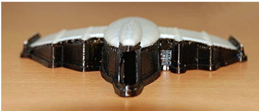
Fig. 12.3 Part printed with soluble support material, courtesy of Joris Peels
