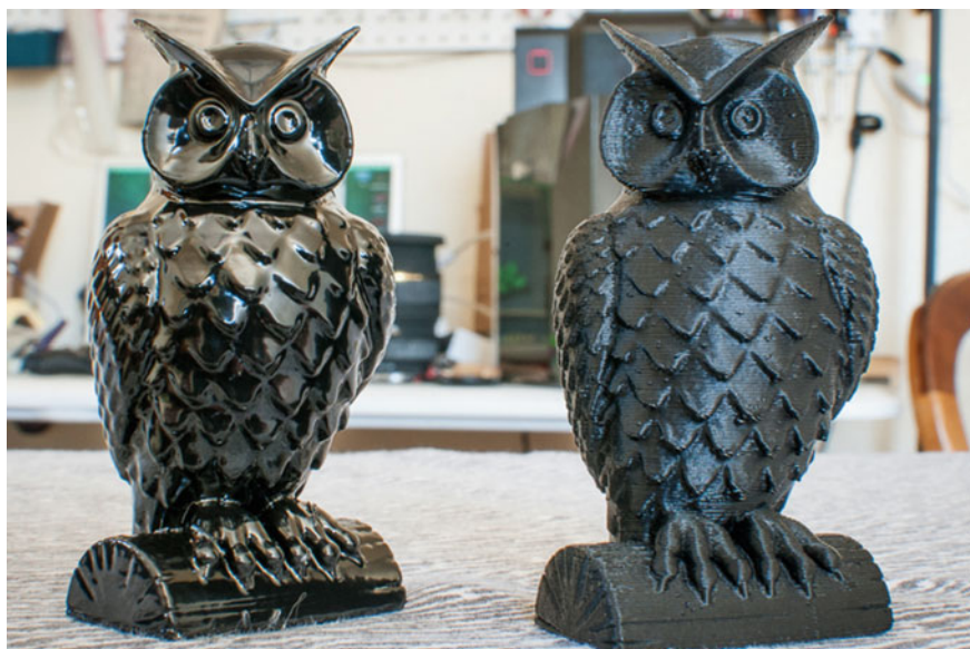
Fig. 12.15 Acetone vapour smoothed ABS parts, courtesy of Andrew Sink
