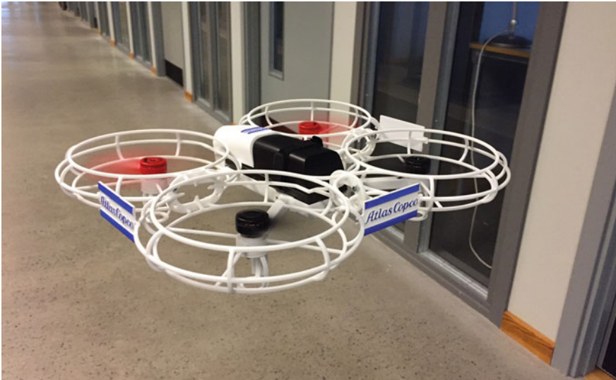
Fig. 1.12 This drone used part consolidation to manufacture the entire drone with only six core components (excluding the company labels). In a larger machine, it could have been made as only two components
