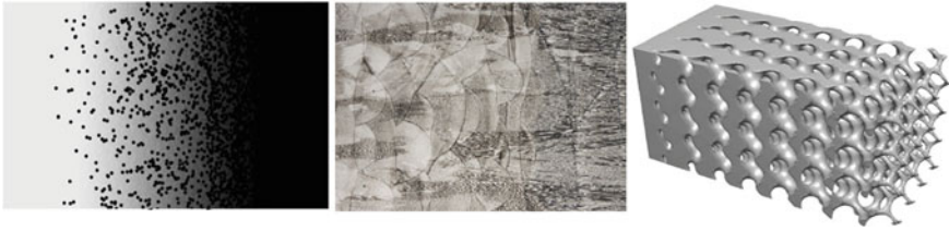
Fig. 13.1 Classification of different types of functionally graded materials, ranging from transitions between different materials to structural geometry changes within the material, courtesy of Mahmoud and Elbestawi [4]
