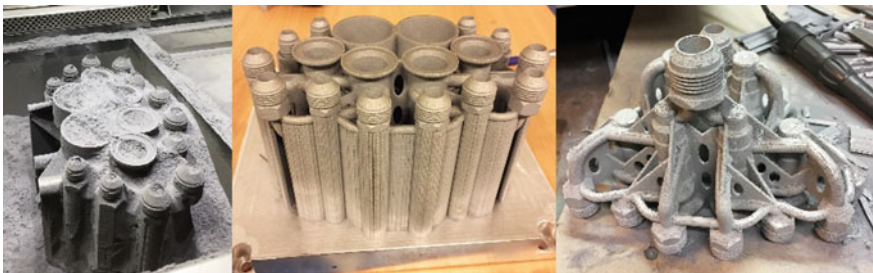
Fig. 3.17 Hydraulic manifold designed for AM with some unremoved powder (left), support structures attached (center), and support material removed (right)
