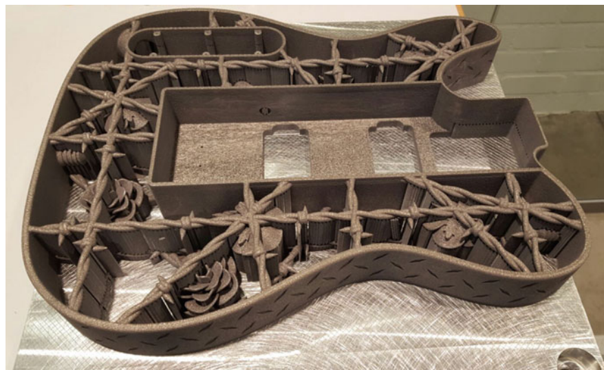
Fig. 12.11 Aluminium guitar still welded to build plate after coming out of the printer, having the loose powder vacuumed away, and being heat treated
