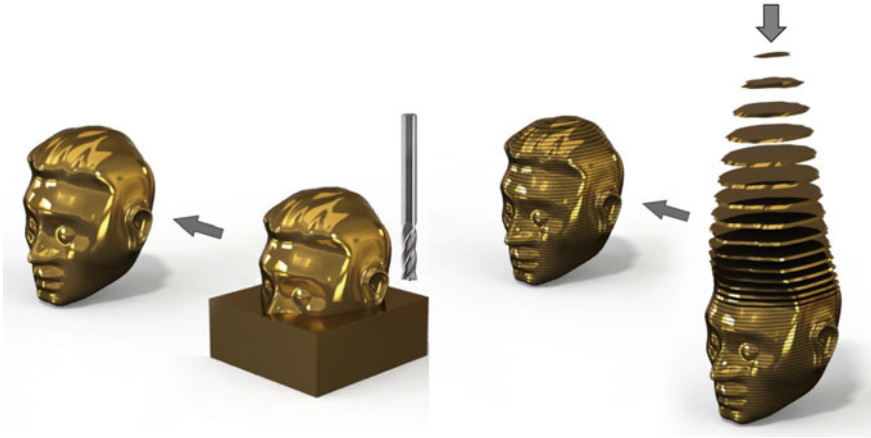
Fig. 1.1 Subtractive manufacturing, where one builds a part by removing material from a block, versus additive manufacturing, in which one builds the part layer-upon-layer
