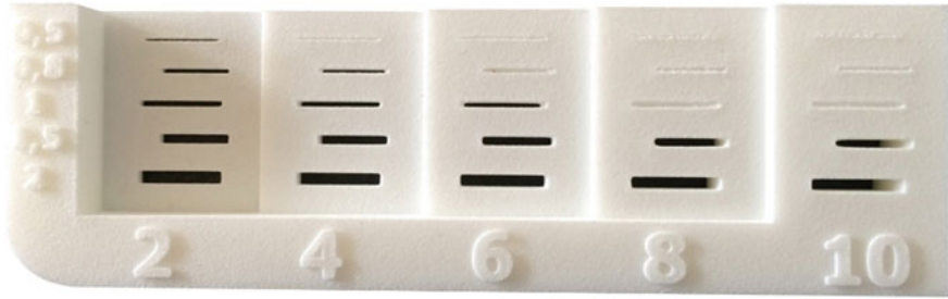
Fig. 3.3 Hole size depends on material thickness
