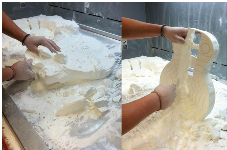
Fig. 12.6 Powder bed fusion parts being removed from the powder ‘cake’
