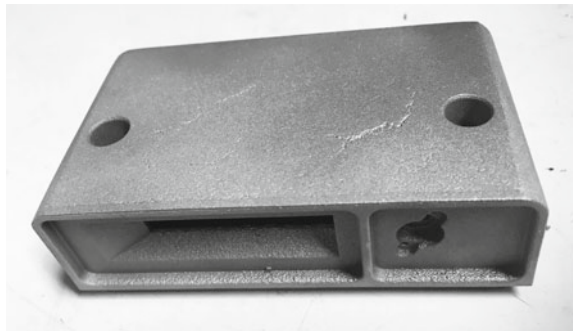
Fig. 9.24 Stress cracks on the bottom of a part printed in a horizontal orientation
