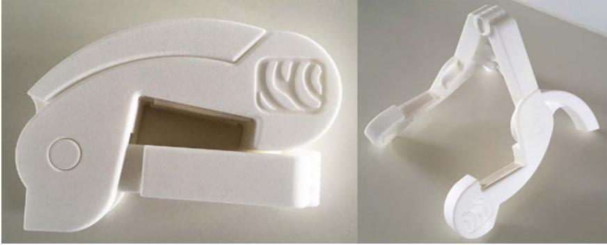
Fig. 1.11 Foldable guitar stand manufactured as a single component using polymer powder bed fusion
