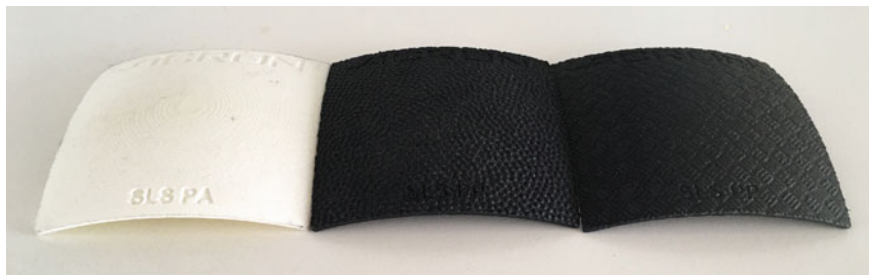
Fig. 12.19 Texturing the curved surface of a part almost entirely eliminates the stair-step effect. The left part clearly shows stair-stepping, whereas the textured parts do not
