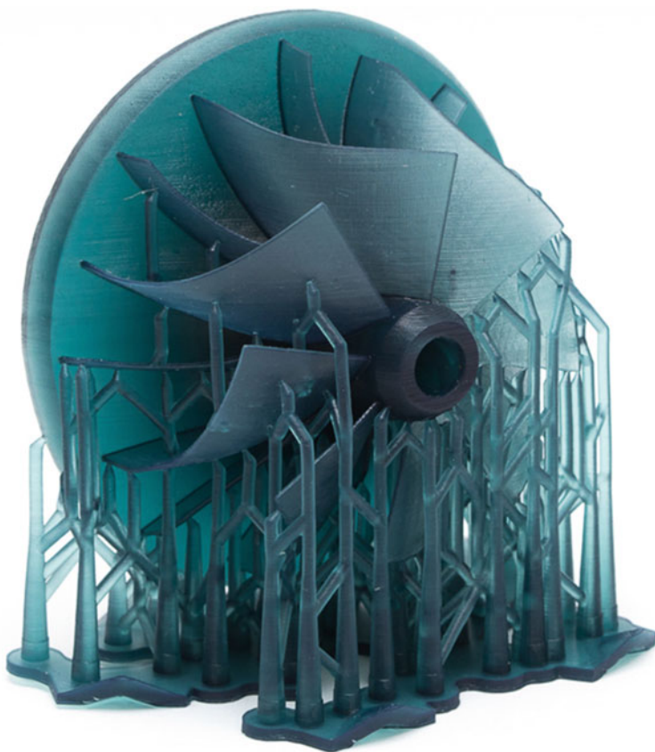
Fig. 12.4 Support material on vat photopolymerisation part, courtesy of www.3dhubs.com
