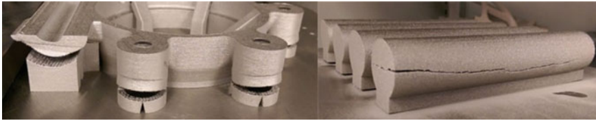
Fig. 9.29 The effect of residual stress on metal AM parts can be strong enough to detach the part from its supports, or to split the part
