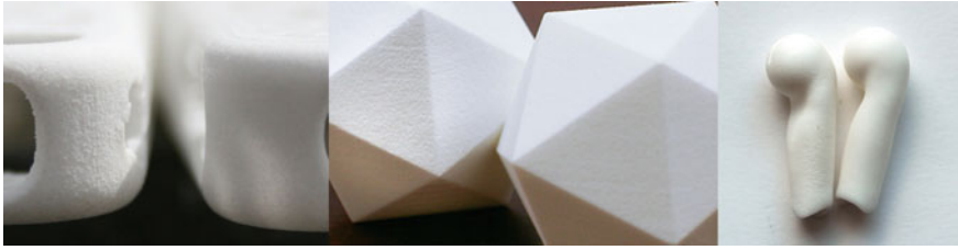
Fig. 12.16 Examples of tumbled AM parts, courtesy of Duann Scott
