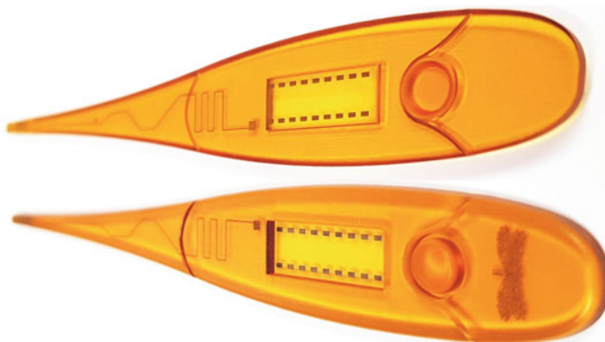
Fig. 13.5 Printed thermometer with printed electronic circuits, courtesy of Nano Dimension
