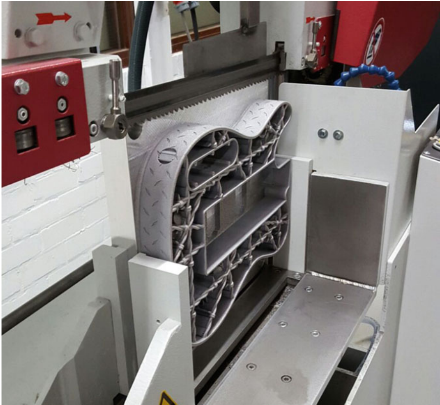
Fig. 12.12 Aluminium guitar being cut off the build plate with a saw
