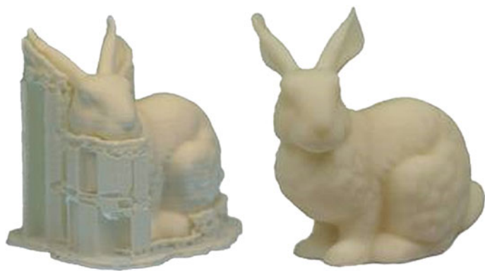
Fig. 7.2 Support material to allow overhanging features to be printed
