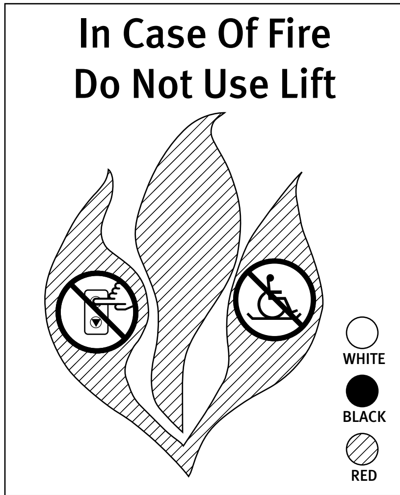
Figure 2.6.7 Platform Lift Corridor Call Station Pictograph
