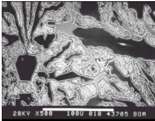
Fig. 2.31. SEM (in backscatter mode) of duplex microstructure. Dense phases (matrix and M_3C carbides) reflect more electrons toward the detector and appear lighter, while less dense phases (e.g., M_7C_3 ) reflect fewer electrons and appear darker. The formation of the peritectic shell of M_3C carbide is shown around most all of the M_7C_3 carbides.
