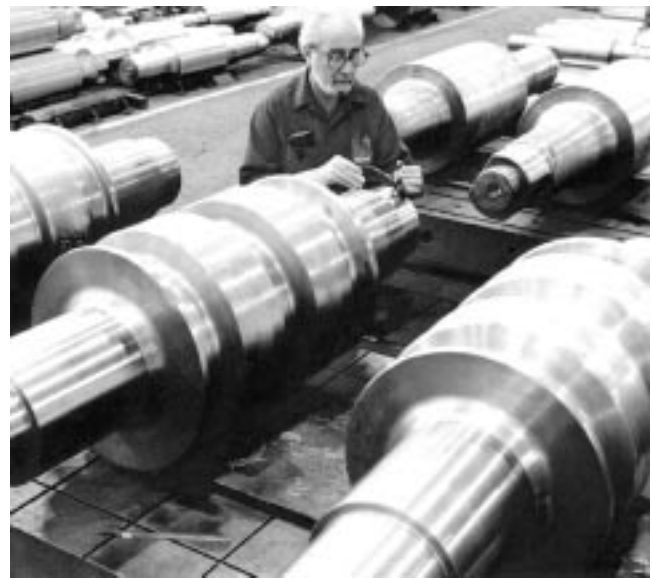
Fig 10.16. Modified Ni-Hard 1 (ASTM IA) mini-mill rolls for the structural steel industry. The roll is statically chill cast. The alloy has been modified to form a mixed microstructure of hard M_3C carbides and spheroidal graphite. (Courtesy of United Foundries)
