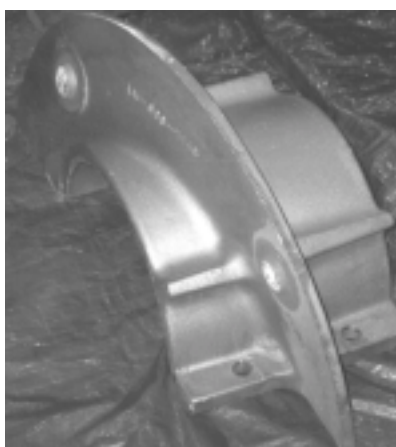
Fig. 10.43b. High-Cr (ASTM IIIA) casting used in asphalt mixing. Casting is approximately 74x46 cm (29x18 in.) and weighs 67 kg (150 lb). (Courtesy of United Machine and Foundry)
