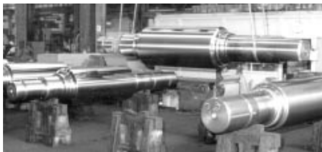
Fig 10.17. High-Cr (ASTM IIB) duplex rolls for hot strip mill applications. The rolls were manufactured by centrifugally casting the high-Cr shell material and then statically casting the body and necks using a gray or nodule iron alloy. The castings shown in the photograph have been heat treated to a shell hardness of around 650 HB and then machined. (Courtesy of United Foundries)
