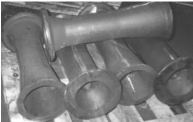
Fig 10.7. Ni-Hard 1 (ASTM IA) nozzles. The approximate weight of one casting is 80 kg (180 lb). (Courtesy of Weatherly Casting and Machine Co.)
