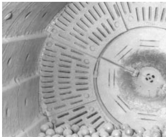
Fig. 10.20. The inside of a ball mill for grinding cement clinker, containing low-C high-CrMo (ASTM IIA) iron balls and liner plates. (Courtesy of IMOA)
