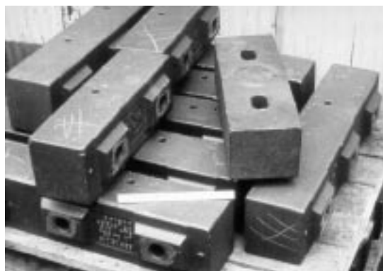
Fig. 10.19. Lifter bars forming part of the lining of an auto-geneous mill, cast of CrMo irons (ASTM IID). (Courtesy of IMOA)
