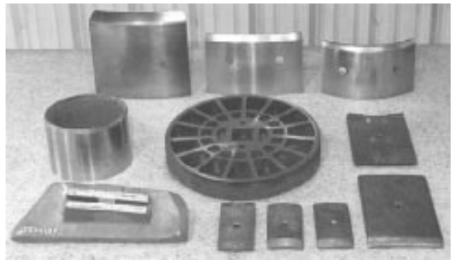
Fig 10.5a. A variety of Ni-Hard 1 (ASTM IA) castings used in aggregate processing, concrete pipemaking, placement and mixing applications. The center mixing wheel is 38.1 cm (15 in.) in dia and weighs about 22 kg (50 lb). (Courtesy of Texaloy Foundry Co.)
