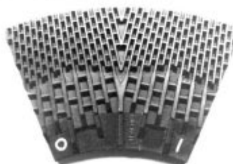
Fig 10.45 High-Cr (ASTM IIIA) AR refiner plates for the pulp and paper industry. The holes are about 35 mm (1.4 in.) dia and the castings weigh about 10 kg (22 lb) each. (Courtesy of Durametal Corporation)
