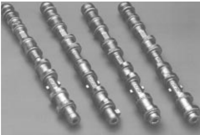
Fig. 10.4. Two-inlet, two-outlet camshafts for BMW 740d 8V cylinder twin-turbo diesel engine, cast hollow in order to reduce weight and save machining costs. The cams are chilled. (Courtesy of BMW)
