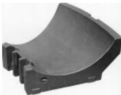
Fig 10.23. High-Cr (ASTM IIIA) wear track segment for coal crushing. The casting weighs approximately 444 kg (1000 lb). (Courtesy of Columbia Steel Castings)
