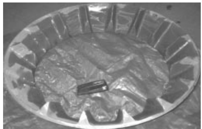
Fig 10.29. High-Cr (ASTM IIIA) casting used to crush sand lumps. Casting is approximately 122x81 cm (48x32 in.) and weighs 89 kg (200 lb). (Courtesy of United Machine and Foundry)
