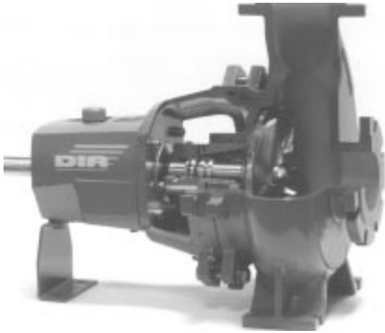
Fig. 10.13. Pump for solids-bearing wastewater with Ni-Hard 1 (ASTM IA) impeller and housing. (Courtesy of DIA-Pumpen)
