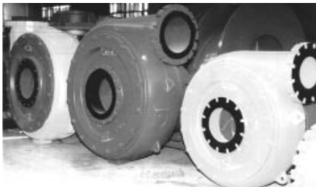
Fig 10.36. High-Cr (ASTM IIIA) sand and gravel pump housings. Casting weights range from 1100 to 2900 kg (2500 to 6500 lb). (Courtesy of Mobile Pulley and Machine Works)
