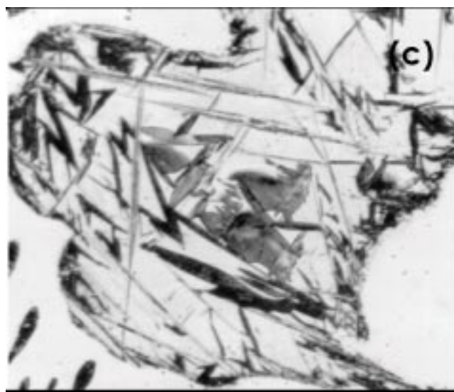
(5.38c) high resolution image of martensite/austenite matrix
