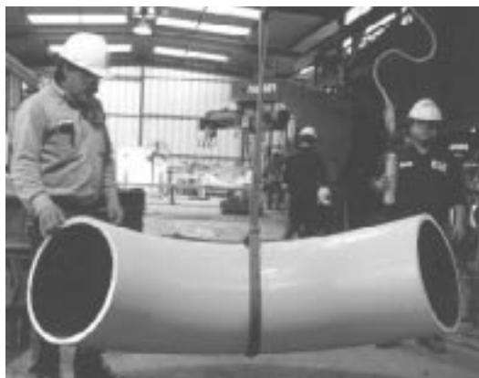
Fig 10.42. High-Cr (ASTM IIIA) pipe elbow to transfer bauxite sludge. The casting has a dia of 53.3 cm (21 in.) and weighs about 550 kg (1235 lb). (Courtesy of Texaloy Foundry Co.)
