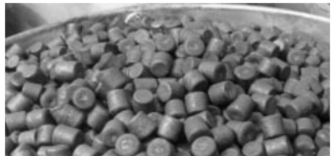
Fig. 10.1. Small grinding media made of chilled white iron. (Courtesy of ZGV)
