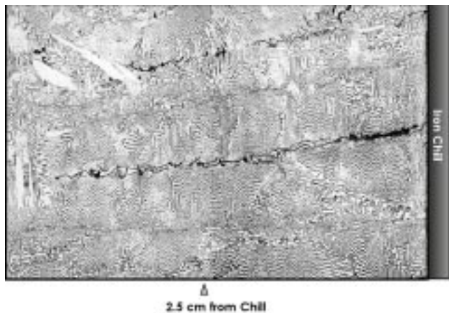
Fig. 2.29. Optical micrograph of a polished section, perpendicular to the chill face. Dark stripes that run perpendicular to the chill face are graphite stringers. General composition is 3.9% C, 0.7% Si and 1.8% Cr. 80X.
