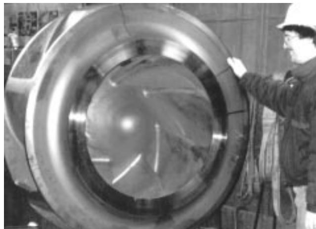
Fig 10.41. High-Cr (ASTM IIIA) 135-cm (53-in.) dia impeller for corrosion/erosion pump slurry application. Casting is positioned on a two-plane dynamic balancing machine. The approximate weight of the casting is 1500 kg (3400 lb). (Courtesy of Weatherly Casting and Machine Co.)
