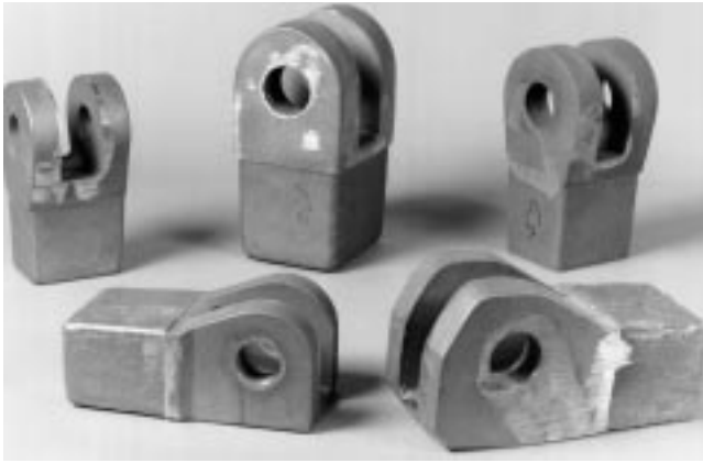
Fig. 10.2. Hammers for brown coal crushers, with white cast iron head cast in a chill mold and gray iron shaft cast in a sand mold. (Courtesy of ZGV)
