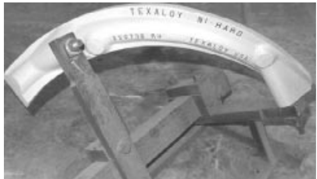
Fig. 10.5b. Ni-Hard 1 (ASTM IA) mixer blade used in concrete mixer (shown on foundry alignment jig). Casting weighs about 191 kg (430 lb). (Courtesy of Texaloy Foundry Co.)
