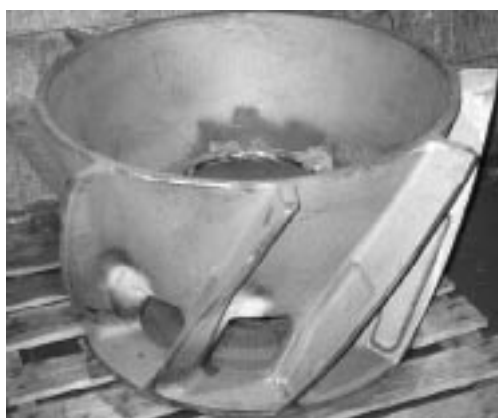
Fig 10.43a. High-Cr (ASTM IIIA) casting used to de-water coal. Casting is approximately 81x81 cm (32x32 in.) and weighs 290 kg (650 lb). (Courtesy of United Machine and Foundry)
