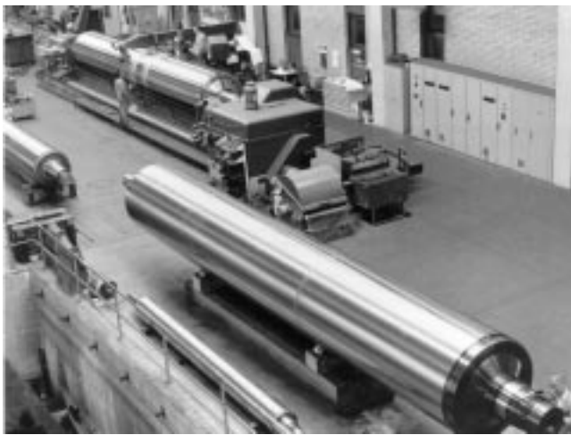
Fig. 10.3. Chilled iron roll for papermaking equipment that is heated from the inside; 65 ton, 1425 mm dia total length 12,300 mm. (Courtesy of ZGV)
