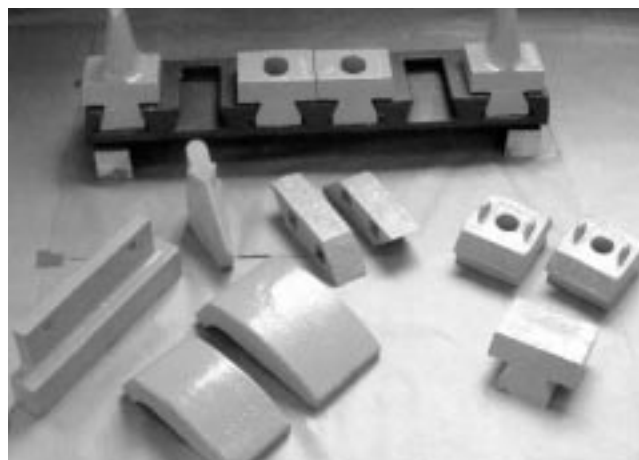
Fig. 10.40. High-Cr (ASTM A532 IIIA) drag head parts for the sand and gravel business. Parts weigh from 15 to 125 kg (~25 to 300 lb). (Courtesy of Mobile Pulley and Machine)
