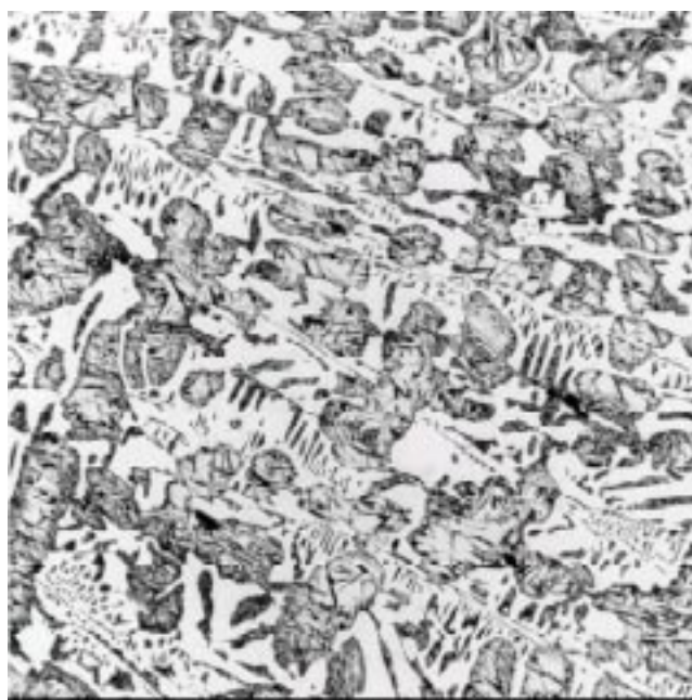
Fig. 1.2. Ni-Hard AR iron showing the eutectic carbides and matrix phases on a 2D plane that was cut through the iron. 500X.
