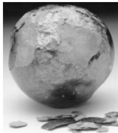
Fig. 8.29. A heavily spalled ball and its detritus after extensive repetitive impacts in the ball-on-ball impact test.
