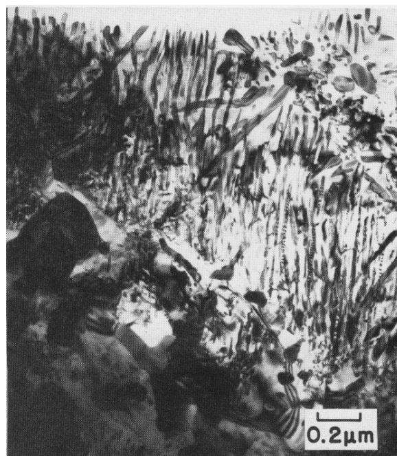
Fig. 3.20. TEM micrograph illustrating fibrous carbides in ferrite in a high-Cr white iron containing 2.9% C-17% Cr-1.4% Mo-1.1% Ni, which was as-cast + subcritically heat treated for two hours at 625C (1160F). (After Biss, 1981)
