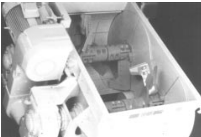
Fig. 10.8. Mixer with blades and lining of Ni-Hard 1 (ASTM IA). (Courtesy of BHS)
