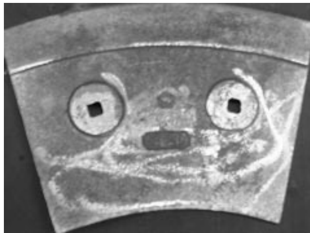
Fig 10.39. An auger flight shoe for a 112-cm (44-in.) Eagle sand screw is shown. This part weighs 5 kg (12 lb) and is cast in the ASTM A 532 Class III Type A. This part is one of approximately 96 pieces that is bolted onto an auger to protect the auger from wear. The screw is designed to wash gravel. (Courtesy of Eagle Foundry Co.)
