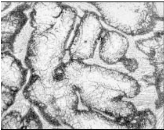
Fig. 1.9. Optical micrograph of a polished and etched surface of a heat-treated 1.1% C, 17% Cr (440C) AR cast iron. The blade-like M_7C_3 eutectic carbides are surrounded by a thin layer of martensite. The very small dots or dark tracings within the ferrite/austenite dendrites are M_{23}C_7 secondary carbides that formed during heat treatment. The light areas are large austenite dendrites. 500X, etched with 2% nital.
