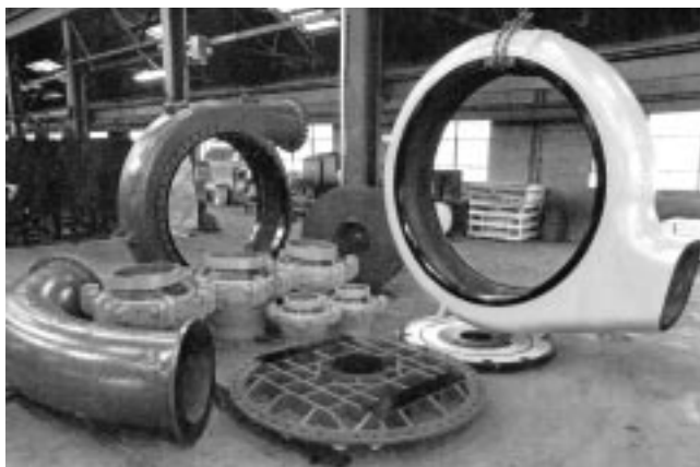
Fig 10.37. High-Cr (ASTM IIIA) AR parts for the dredging industry. Weights of large castings can exceed 5780 kg (13,000 lb). (Courtesy of Mobile Pulley and Machine Works)
