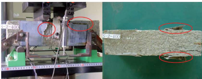
Figure 3. De-lamination of CFRP at failure
