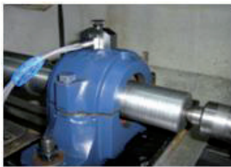
Figure 6. AE sensor mounting on the bearing housing with a magnetic clamp
