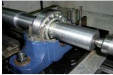
Figure 3. Test bearing arrangement on the housing, locating rings, and others equipments
