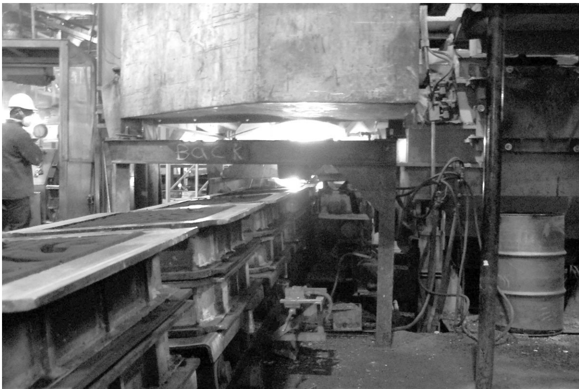
Fig. 6-11. Automatic pressure pouring of indexed mold stack are shown. (Artwork courtesy of Sloan Valve Company, USA)
