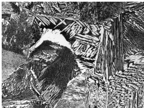
Fig 10-5. Microstructures from alloy C85800 cast in permanent mold showing the dendrite morphology (left) before, and (right) after grain refinement with boron (100x). (Artwork courtesy of CanmetMATERIALS, Hamilton, ON, Canada.)
