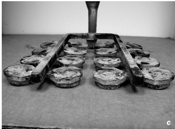
Figs. 7-19a, b & c. These three photos illustrate a kiss gated pattern system for a valve cap. (Artwork courtesy of Ford Meter Box).
