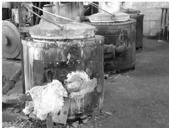
Fig. 4-2. A battery of gas-fired, lift-out crucible furnaces is shown. (Artwork courtesy of Cochran Foundry, York, PA.)
