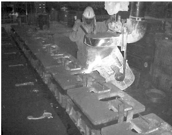
Fig. 6-7. Pouring bronze castings from a ladle shell lined with graphite; teapot-type liner providing skimmer and bottom-pour tube. (Artwork courtesy of Fresno Valves and Castings, Inc., USA.)
