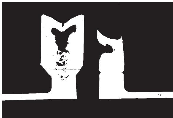
Fig. 13-9 Two types of shrinkage characteristics of the cupronickel alloys are illustrated above: piping and interdendritic.
