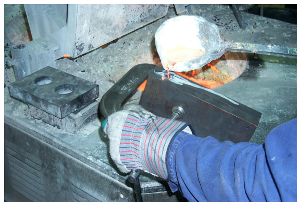
Fig. 3-20 (a & b). Hand pouring of a permanent mold casting. Note the tilted position of the mold in view b. (Artwork courtesy of Sloan Valve.)
