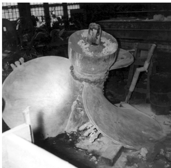
Fig. 3-7. A bronze propeller is shown at shakeout, cast in a cement-bonded mold. (Artwork courtesy of Columbian Bronze Corp., Freeport, NY)
