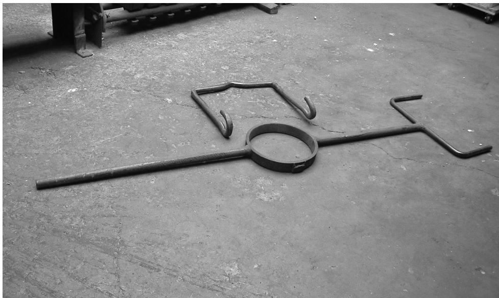
Fig. 6-3. A pouring shank with a support ring for use with crucibles in push-out or lift-coil induction furnaces is shown. (Artwork courtesy of H. Kramer & Co.)
