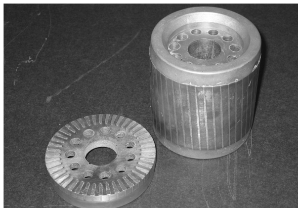
Fig. 3-18. An aluminum “squirrel cage” for a small motor after dissolution of the iron in nitric acid. (Artwork courtesy of Copper Development Association.[ www.copper.org ])
