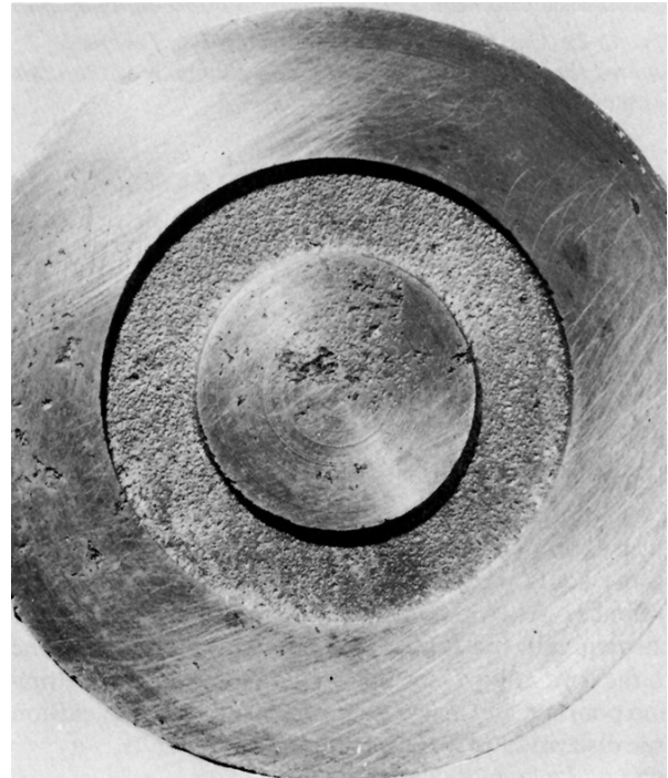
Fig. 15-31. A brass disc, 200 mm (8 in.) in diameter, containing dross inclusions is shown.
