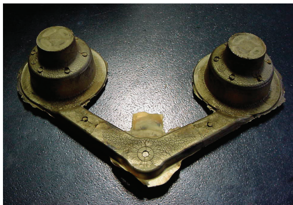
Fig 3-13(a & b). A diecast component showing the fixed and moveable die sides of the casting. (Artwork courtesy of the Kohler Company.)
