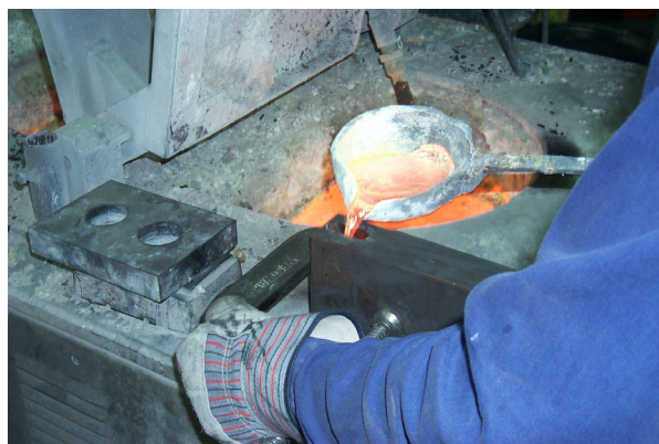
Fig. 3-20 (a & b). Hand pouring of a permanent mold casting. Note the tilted position of the mold in view b. (Artwork courtesy of Sloan Valve.)
