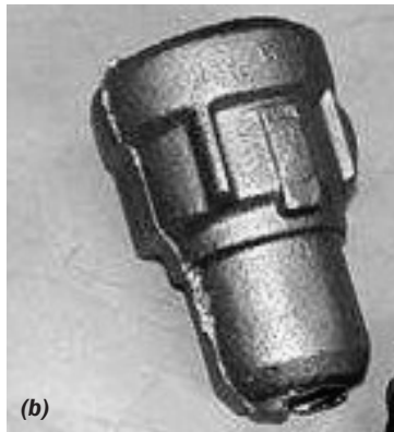
Fig. 3-2. Shown are typical green-sand cope and drag halves of a mold (a), along with the casting produced from the mold (b).
