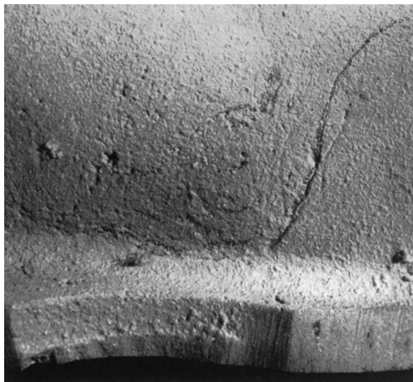
Fig 15-32. This casting is shown exhibiting oxide film inclusions. The metal entered the mold with turbulence and aluminum oxide skins were trapped in the casting wall.
