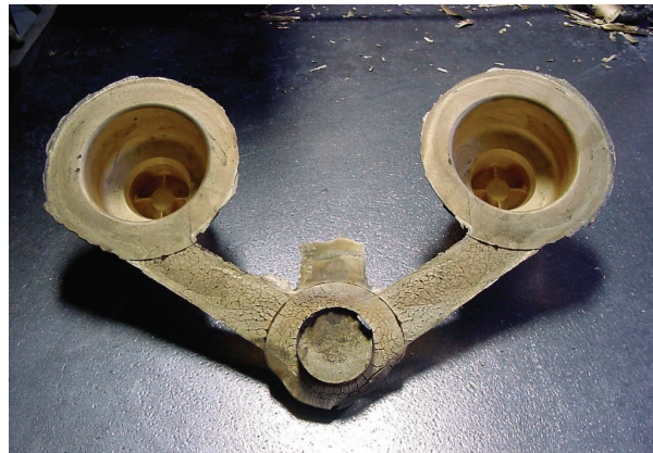
Fig 3-13(a & b). A diecast component showing the fixed and moveable die sides of the casting. (Artwork courtesy of the Kohler Company.)
