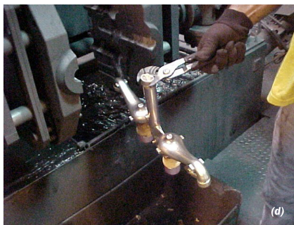
Fig. 3-22. A low pressure permanent mold casting machine, view (a) for copper and views (b-d) show the sequence of operations [Artwork courtesy of CANMET (view a) and Kohler (views b-d)]
