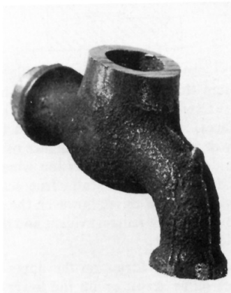
Fig 15-22. These castings are shown with burn-on.
