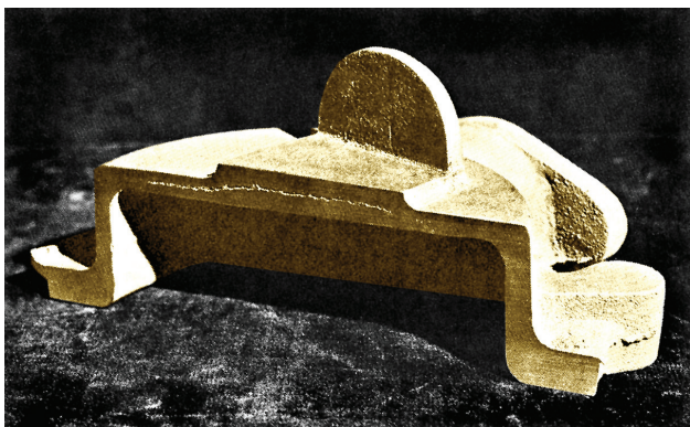
Fig. 8-1. Brass sand casting shows centerline shrinkage crack. Lowering iron and tin content, increasing riser size and reducing pouring temperature would eliminate the shrink.
