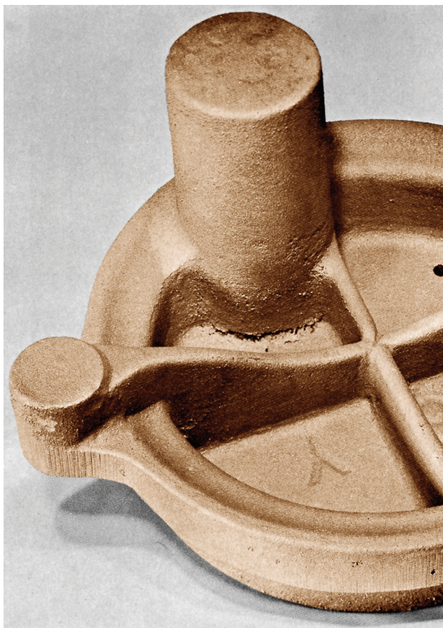
Fig. 6-1. Bronze alloy in dry sand that shows shrinkage extending to surface as a hot tear.
