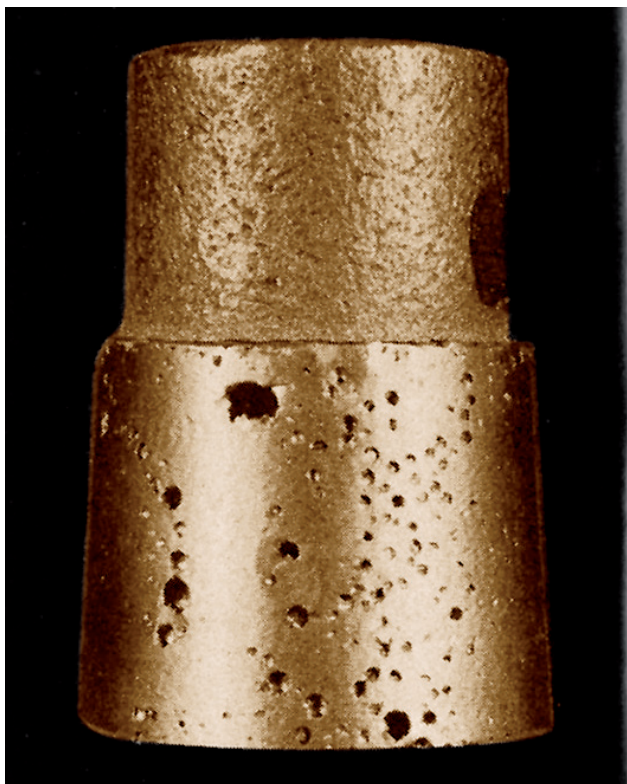
Fig. 7-5. Bronze stopper cast in green sand has blowholes due to gassy melt and/or mold/metal reaction with excessive residual moisture in the sand.
