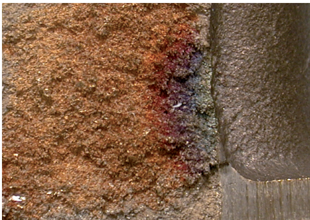
Fig. 7-9. A discoloration and porosity in red brass is due to gas evolution and high pouring temperature.
