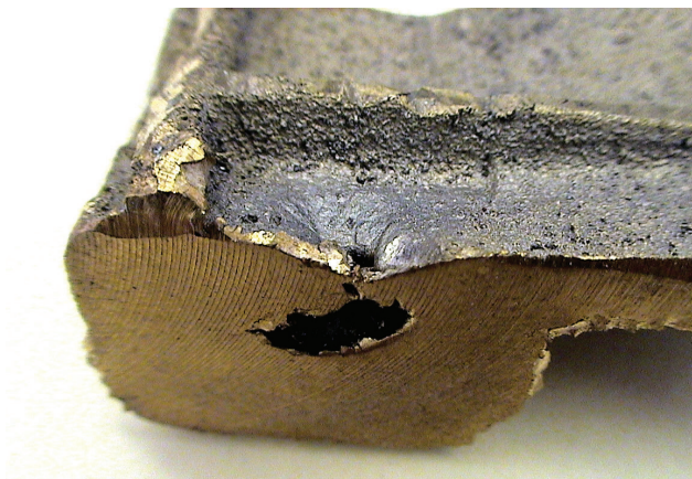
Fig. 7-13. A core gas blow in leaded red brass is the result of poor venting and pouring temperature being too high. Also, inadequate gating causes localized heating at a thick section and a concentrated gas blow within the casting.
