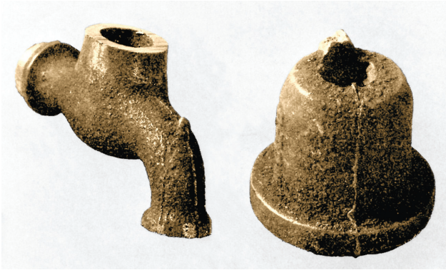
Fig. 9-1. A bronze alloy in green sand exhibits burn-on.
