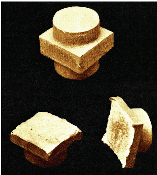
Fig. 5-1. A bronze screw nut cast in green sand shows effects of interrupted pouring.
