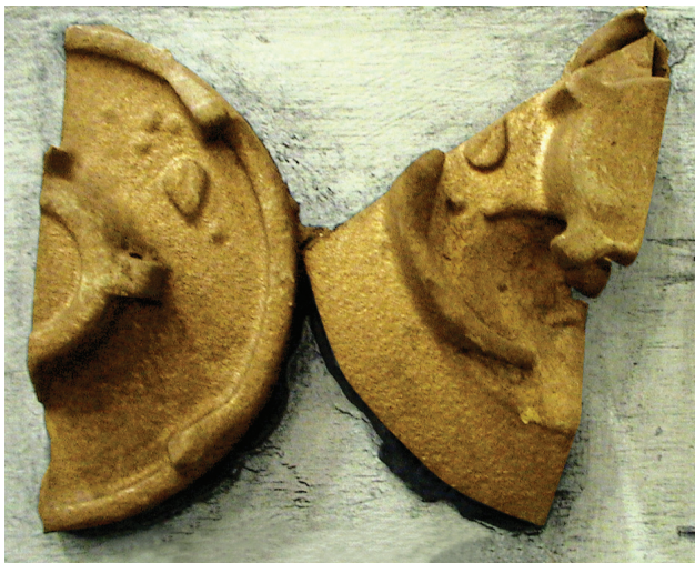
Fig. 11-6. Overblast damage on brass casting is due to excessive shot or grit casting cleaning.
