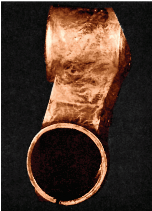
Fig. 2-2. Same casting as in Fig. 2-1 shows flow marks caused by high pouring temperature and turbulent filling of the mold.
