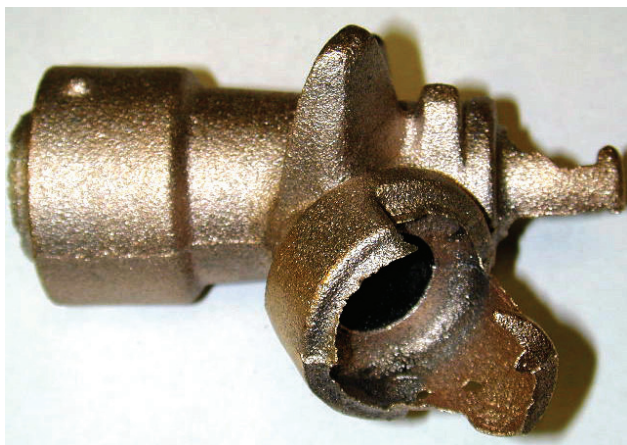
Fig. 4-16. Improper core alignment in red brass
