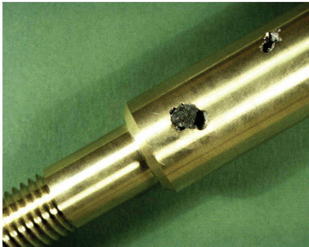
Fig. 10-6. A macro-inclusion in brass casting is a possible refractory vessel erosion.
