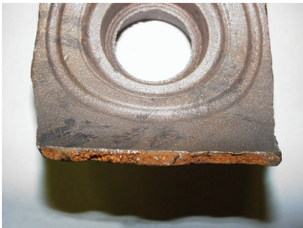
Fig. 6-5. Hot tear in red brass caused by shakeout, which is too soon and/or too hot.
