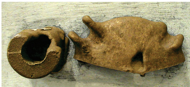
Fig. 5-8. A misrun in red brass is caused by low temperature, inadequate gating and low phosphorus deoxidation.
