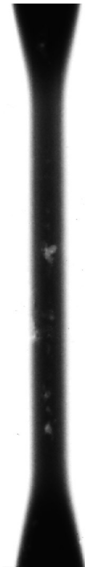
Fig. 7-10. X-ray of cast test bar exhibits gross porosity in brass.
