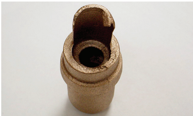
Fig. 4-2. Core crush from insufficient core strength
