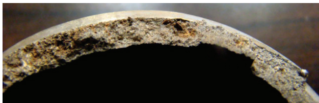
Fig. 8-5. Shrinkage porosity in red brass is caused by poor solidification (low pouring temperature, inadequate feeding).
