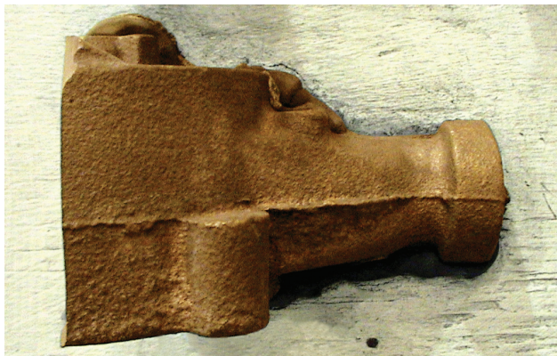
Fig. 4-10. Sticker is caused by poor sand molding and pattern problems
