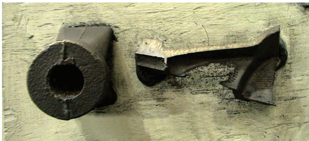
Fig. 1-4. The broken core shows low binder content, poor density and age.
