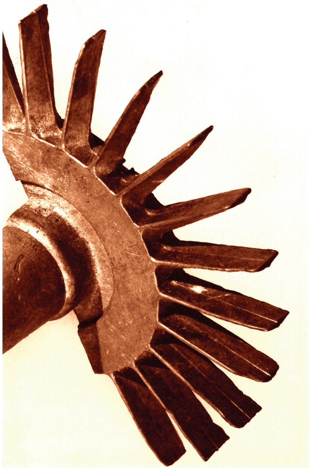
Fig. 5-2. A cupro-aluminum permanent mold casting exhibits a misrun due to lack of venting.
