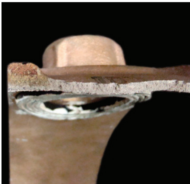
Fig. 8-8. Casting shows shrinkage from inadequate ingate solidification.
