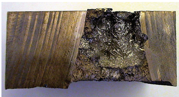
Fig. 8-7. Shrink in semi-leaded red brass resulted from incorrect pouring temperature and inadequate risering.
