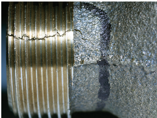
Fig. 11-5. Lead-free brass casting, cracked during machining, is caused by severe stress and heat.
