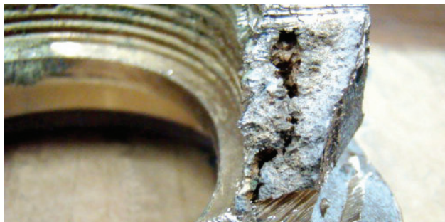
Fig. 8-3 Centerline shrinkage in red brass is caused by insufficient feeding.
