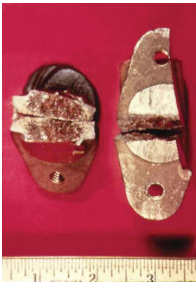
Fig. 1-1. Aluminum in red brass is an impurity that results in casting micro-structural weakness prone to cracking.
