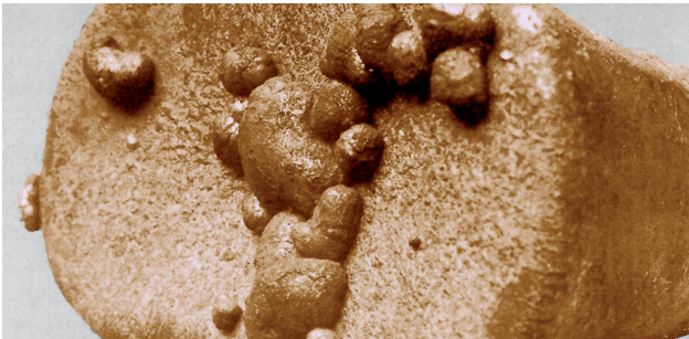
Fig. 11-1. Leaded tin bronze cast in green sand. Sprue exhibits tin sweat.
