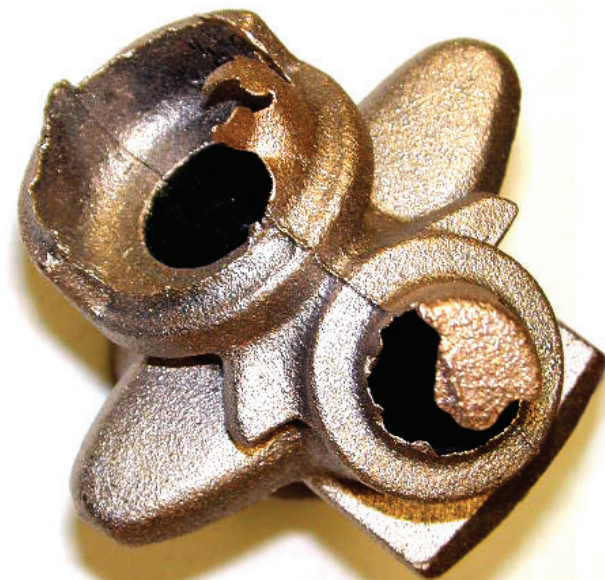
Fig. 5-10. A dimensionally incorrect red brass casting due to core shift.
