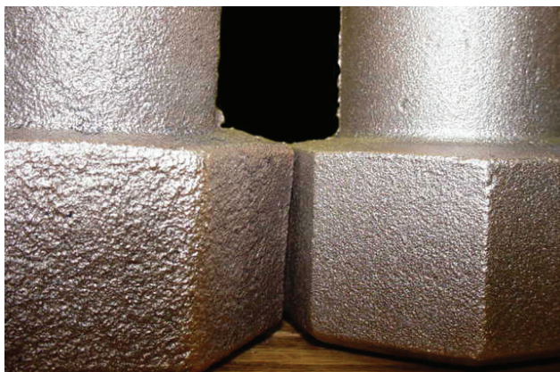
Fig. 4-13. Rough surface on red brass is due to wet sand (moisture too high).
