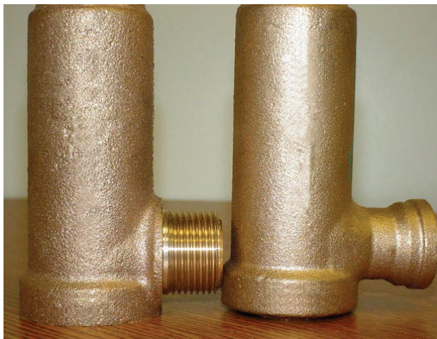
Fig. 4-14. Rough surface on red brass is due to too coarse grain fineness distribution.
