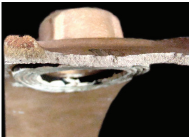
Fig. 5-5. Unsatisfactory ingate solidification in leaded red brass.
