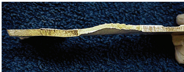
Fig. 1-3. The yellow brass handle, cast in green sand, exhibits unusually large dendritic growth. This is evidence of a melt and/or pour temperature, which is too high, and also of zinc flaring.
