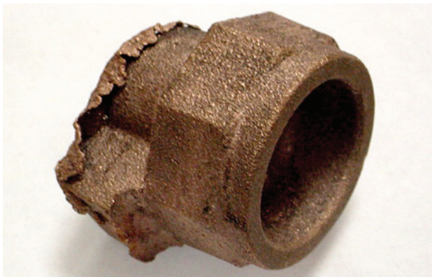
Fig. 4-5. Swell is caused by cracked sand mold in red brass (C83600).
