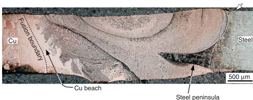
Figure 21.3 A transverse macrograph showing a Cu-to-steel arc weld showing three features associated with the resulting macrosegregation between these dissimilar metals; i.e. a steel peninsula (at the right in the image), an irregular-shaped Cu-beach (at the left in the image), and a layered weld metal (in the bulk of the fusion zone). Source: Soysal et al. (2016). Used under reciprocal agreement between Wiley and Elsevier for fair use.
