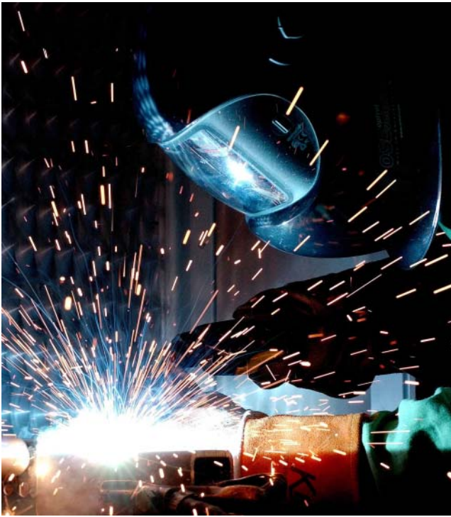
Figure 8.11 Photograph showing sparks from globules of molten metal known as “spatter,” typical of some welding process conditions. Here, gas-metal arc welding (GMAW) is being performed. Source: Photograph by William M. Plate, Jr., for the U.S. Air Force, as ID 040112-F-16633-001, 12 January 2004. Freely used from the public domain as the work of an employee of the U.S. government.
