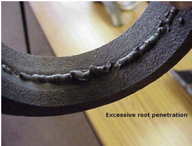
Figure 8.6 Photograph showing excessive root penetration in a fusion weld to create what are variously called “icicles,” “grapes,” or, in the vernacular, “dingle-berries.” Source: Khichade (2015). Used with permission of KEC International Ltd., Mumbai, India.
