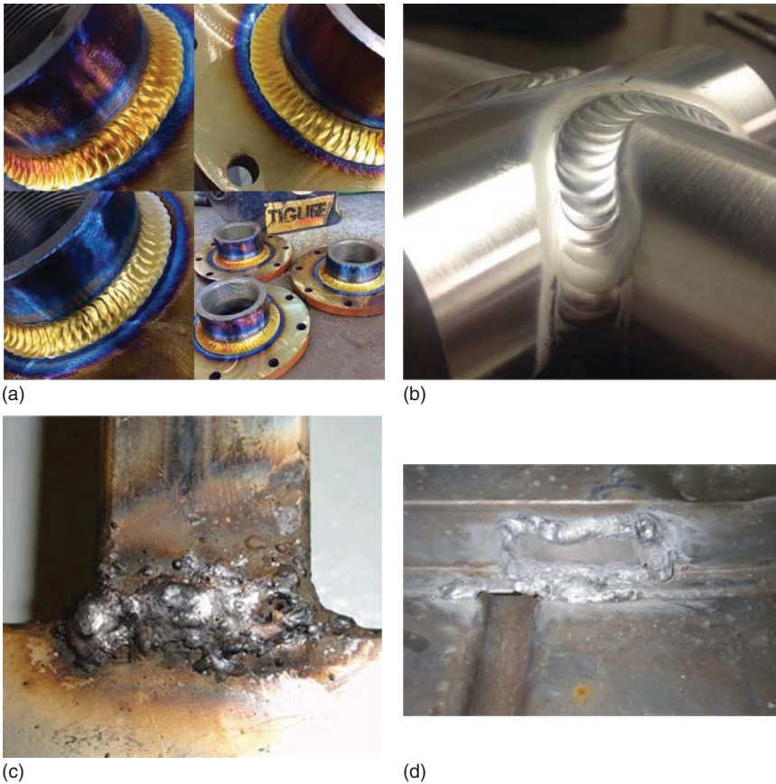
Figure 1.3 Two examples of superbly made fusion arc welds using manual gas tungsten arc (TIG) welding in (a) steel fittings and (b) Al alloy bicycle frames. In addition, two badly made welds: using a gas-metal arc to repair (c) a steel automobile part and (d) an Al alloy boat structure at a factory repair shop, with neither source being identified – fortunately for them – as images are in the public domain! Source: The former by Scott Raabe at his Clean Cut Metal Works, Houston, TX, USA and used with his kind permission; and the latter on the website www.cycling.zanconato.com by Mike Zanconato at Zanconato Custom Cycles, Sutton, MA, USA and used with his kind permission.
