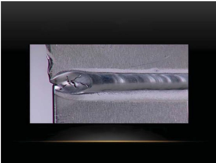
Figure 6.4 A photograph showing a crater crack caused by insufficient filling at the end of a weld. Source: TWI (2015). Used with permission of TWI.
