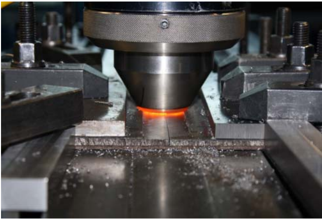
Figure 14.2 Photograph showing a friction stir weld being made in difficult-to-weld oxide-dispersion strengthen (ODS) steel. Source: The Welding Institute (2016). Used with permission of TWI Ltd.
