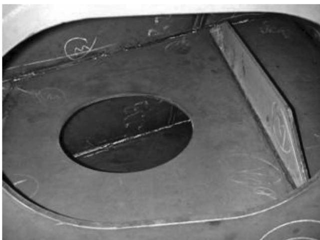
Complex structure, with lower welds only accessible through the hole.
