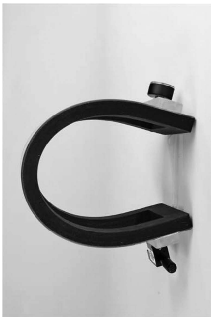
Flex box for testing welds on a radius
