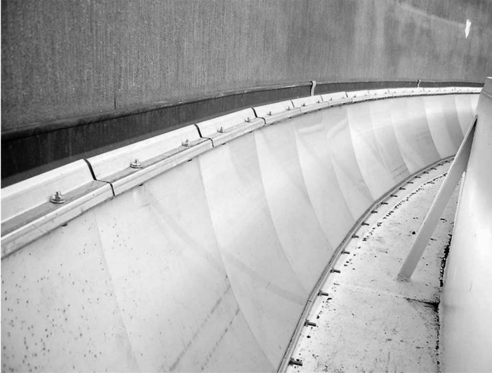
Pantograph-type mechanical shoe seal.
