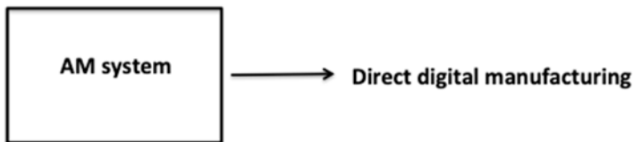
Fig. 9.6 DDM because of confinement of process within one system and no need of post-process
