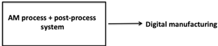
Fig. 9.5 DM because of one system confining both process and post-process but not DDM because of presence of two processes (one process and one post-process)
