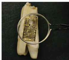
Graphene wireless sensor biotransferred onto the surface of a tooth
