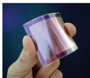
Solar panel films incorporate nanoparticles to create lightweight, flexible solar cells.
