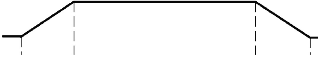
Fig. 4.7 Slope current control during start and stop [8]
