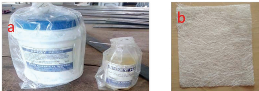
FIGURE 16.1 Composite Raw Materials: (a) Epoxy Resin (LY 556) and Hardener (HY951) and (b) E-Glass Fiber
