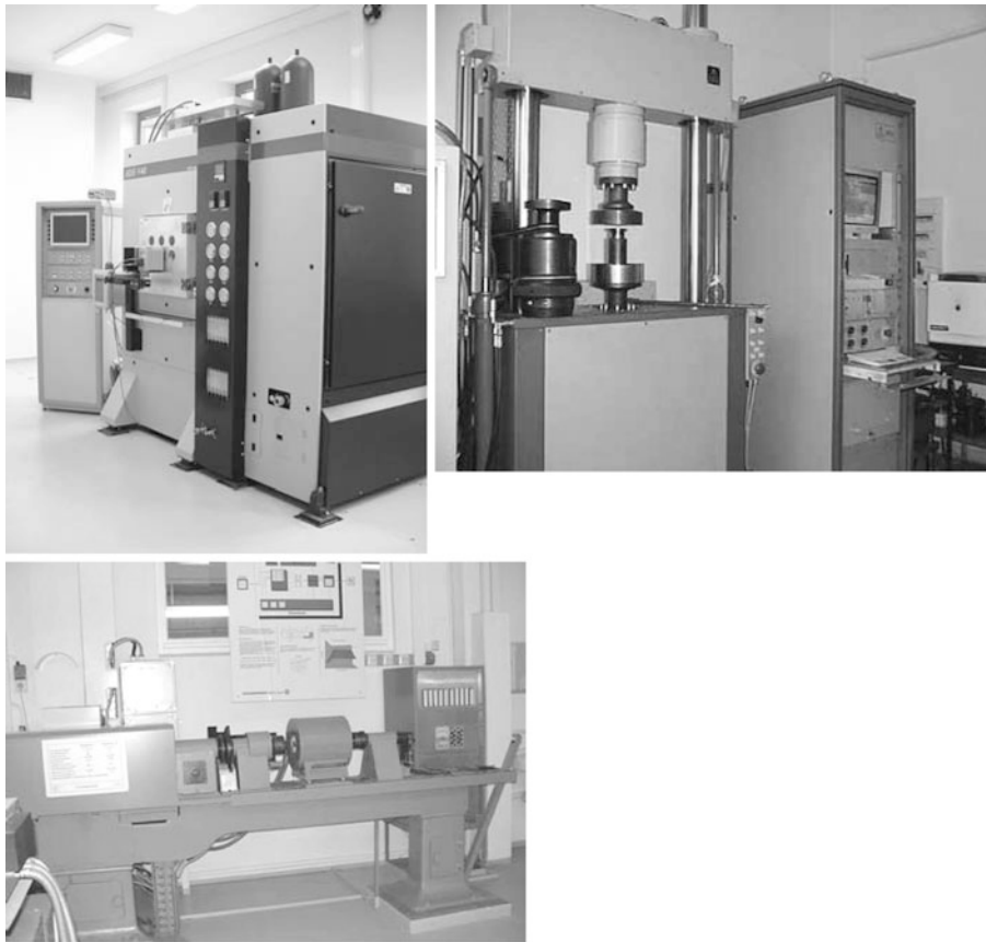
Fig. 1.5a Testing systems. Gleeble HDS-V40 (upper left). Servo hydraulic HDS 40 (upper right). Torsion plastometer (left)
