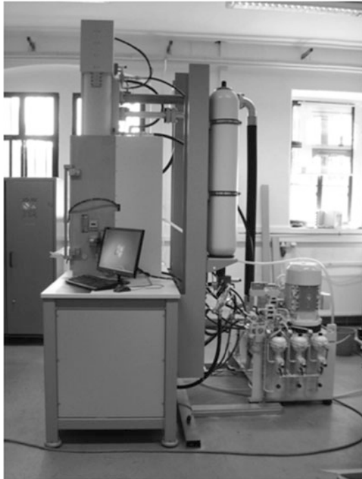
Fig. 1.5b Multidirectional metal forming simulator BÄHR MDS 0830
