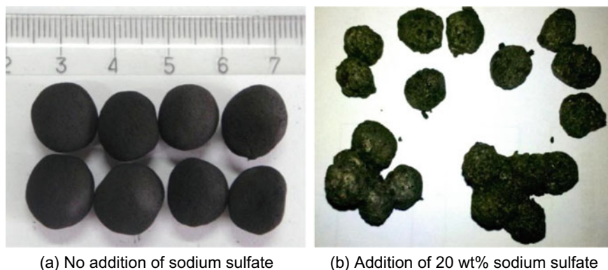
Fig. 2.33 Appearance of reduced pellets of laterite ore (1100 °C, 60 min)
