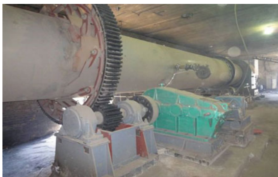
Fig. 2.64 Coal-based rotary kiln for the industrial test
