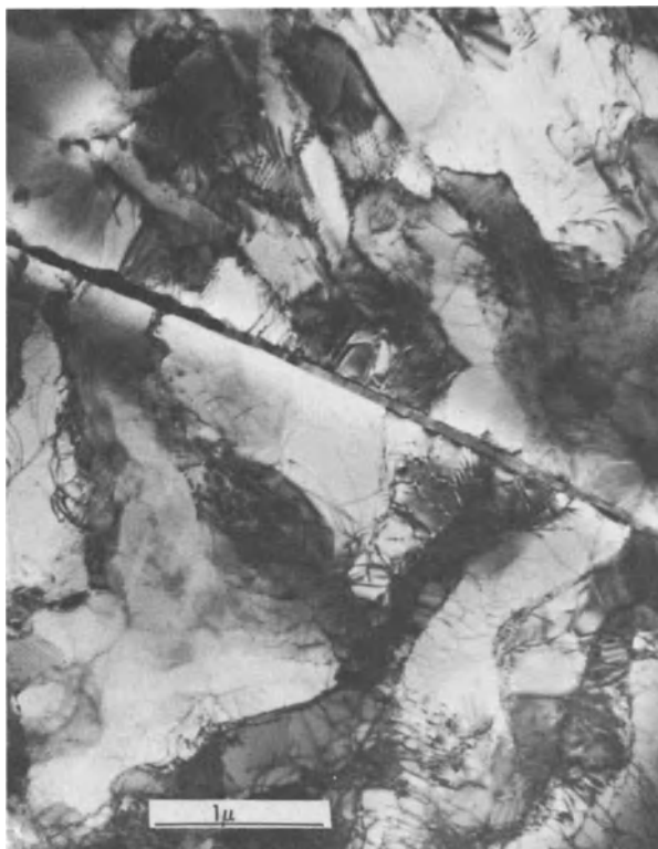
Fig. 83. Grain-boundary precipitates in an Al-8% Mg alloy that was cold worked 20% and annealed in region C of Fig. 77.
