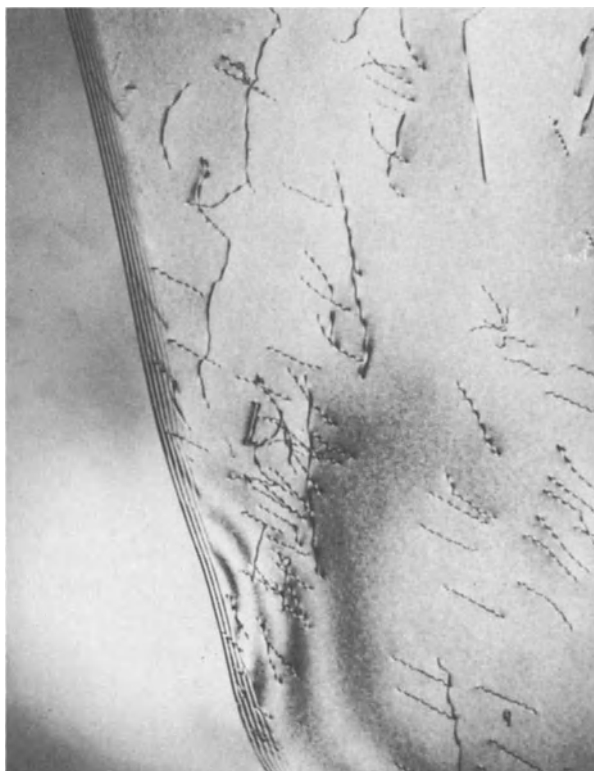
Fig. 82. Precipitate-free grain boundary in an Al-8% Mg alloy after air cooling from the single-phase \alpha field.
