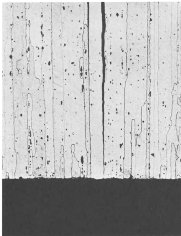
Fig. 4. Typical intergranular stress-corrosion crack in 0.25-in.-thick 7075-T651 plate stressed in the short transverse direction.
