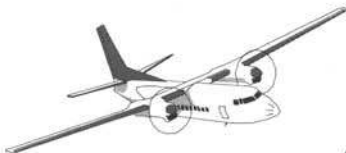
High-wing commercial/military transport 2 \times 1750 hp (1505 kW) turboprop
