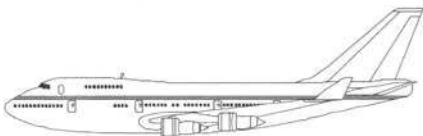
B747-400 long-haul airliner 4 \times 58\,000 lbf (258.6 kN) turbofan
