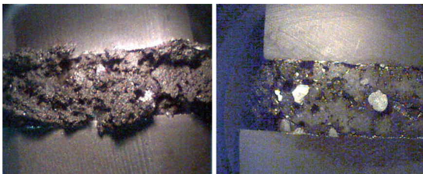
Fig. 3.85 Appearance and thin sections of ore-coke briquette No. 2 with a Penolite binder after determining the hot strength (on the left is a briquette; on the right is a thin section, magnification 10). The composition of the briquette—Kazakhstan chrome ore, coke breeze—8% by weight of ore, and Penolite in the amount of 6% by weight of the ore, drying at room temperature for 24 h. The experimental conditions are linear heating of the sample at a rate of 17 °C/min to a temperature of 1780 °C under a load of 2 kg in a reducing atmosphere
