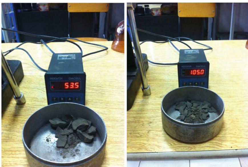
Fig. 3.88 Briquette No. 5 after splitting (left) and compressing (right)
