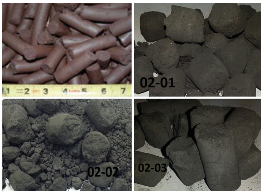
Fig. 3.96 Raw (top left) and reduced brex after extraction from steel packages
