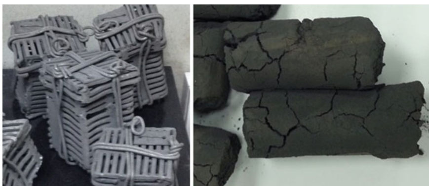
Fig. 3.97 Rigid steel baskets for charging brex into the Midrex reactor (left) and the appearance of brex on the cement binder after removal from the reactor
