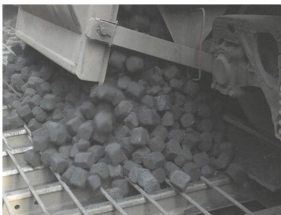
Fig. 3.33 Unloading of vibropressed briquettes from the car
