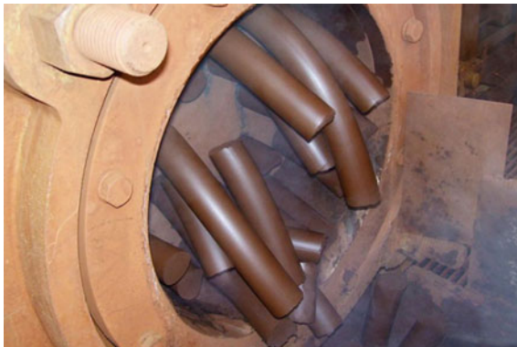
Fig. 3.14 Extrusion briquette manufacturing in Colombia
