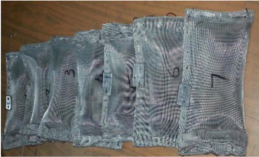
Fig. 3.94 Steel baskets for charging brex together with pellets into a Midrex reactor
