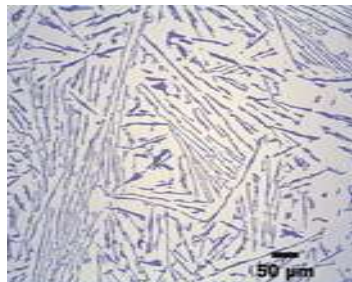
Al – 12% Si, as-cast, near eutectic, "Si Blue" etch
