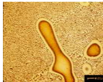
Na-Modified Al – 12% Si, as-cast, near eutectic, Weck's Reagent, Polarized Light
