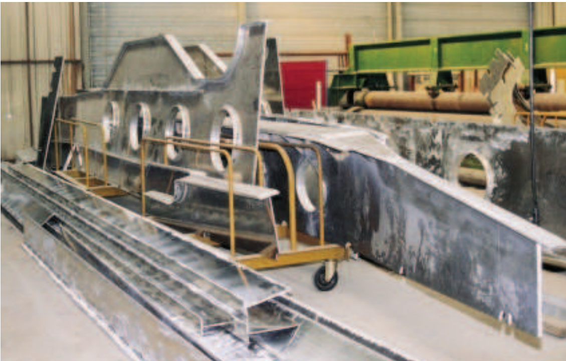
HIGH INERTIA BEAM FABRICATED BY WELDING SHEETS
