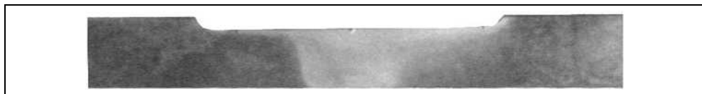
Fig. 1. Typical image of a weld obtained by FSW.
