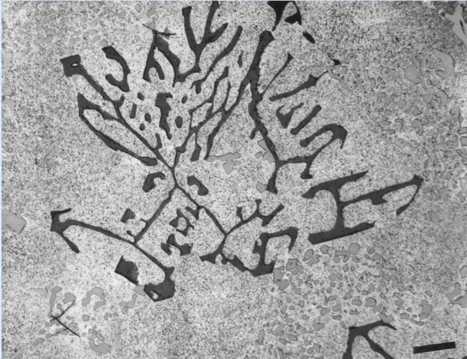
As-cast A356 aluminum (Al – 7% Si – 0.3% Mg – <0.2% Fe) etched with Keller’s reagent. Magnification bar is 20 \mu\text{m} long.
