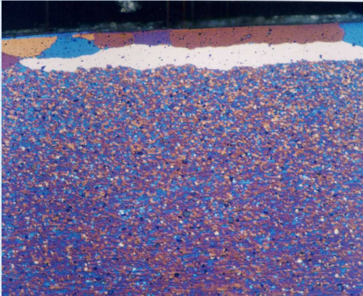
Wrought 7075-T74 aluminum (Al – 1.6% Cu – 2.5% Mg – 5.6% Zn – 0.23% Cr) anodized with Barker's reagent (20 V dc, 2 min.) showing highly elongated, recrystallized surface grains on a fine grained interior structure. Magnification bar is 50 μm long. Viewed with crossed polarized light plus sensitive tint.
