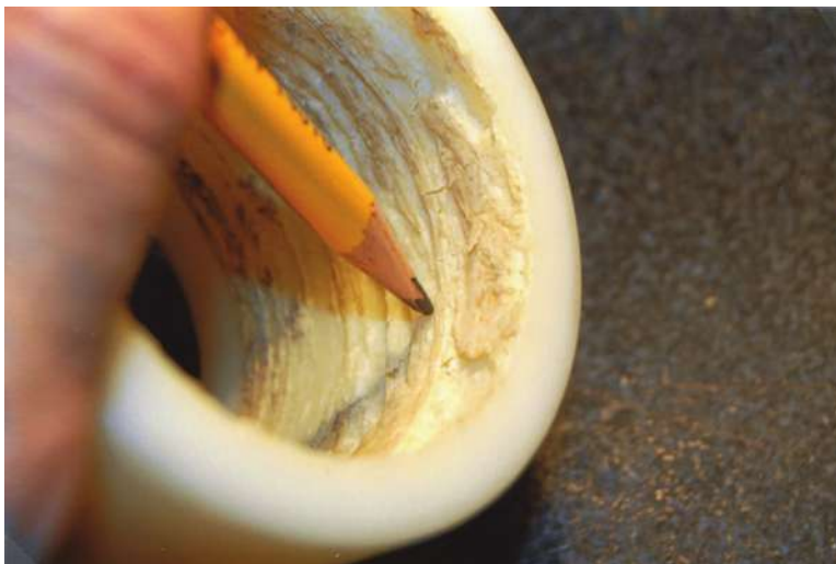
COLOR FIGURE 3.20 Bore of a plastic bushing after a temperature-induced seizure.
