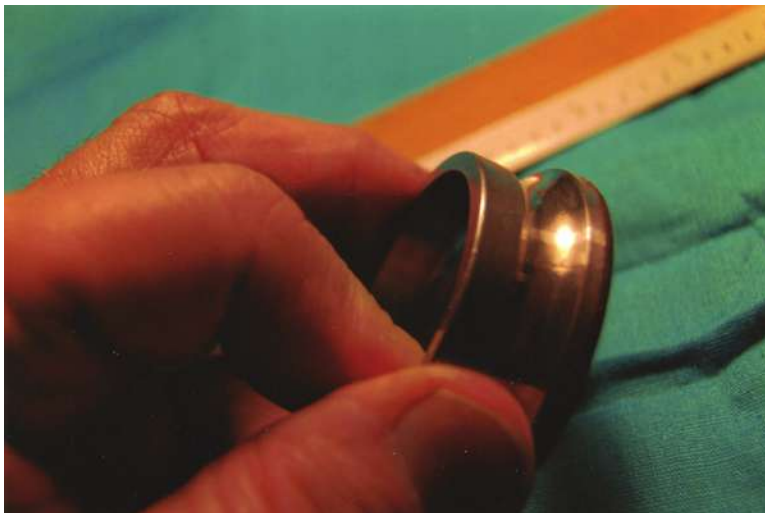
COLOR FIGURE 5.8 Brinelling of a raceway from static overload.
