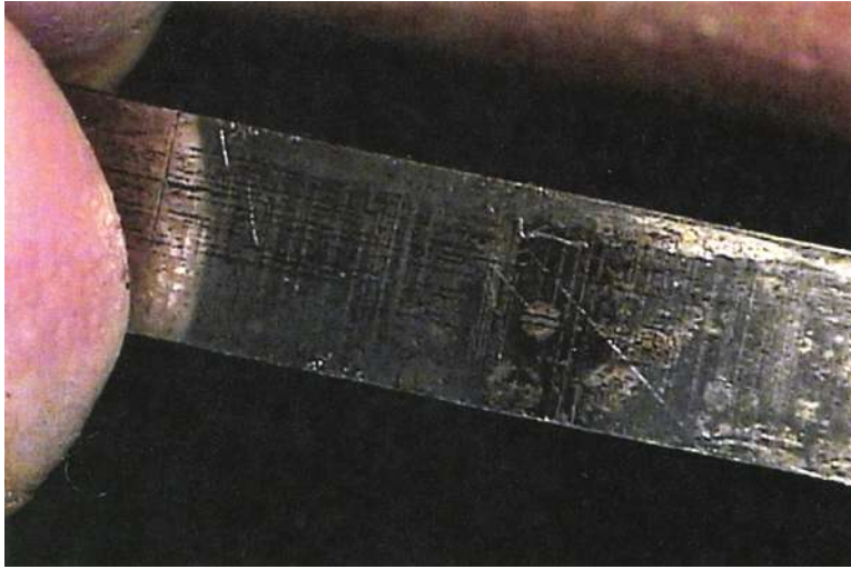
COLOR FIGURE 7.14 Mild wear on a piston ring.
