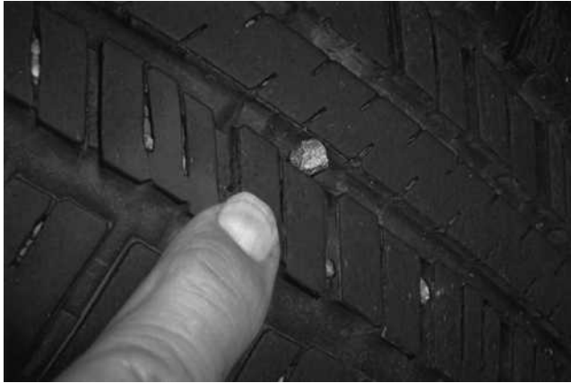
FIGURE 4.21 Abraded rubber on an automobile tire.
