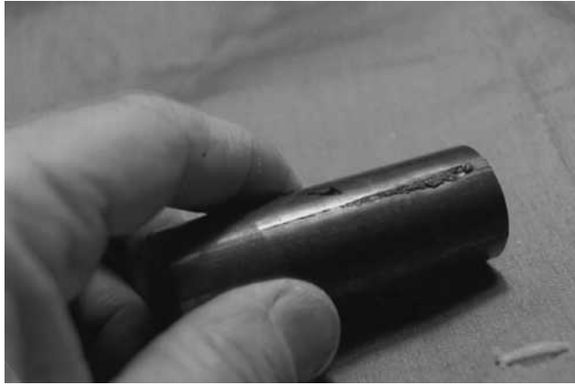
FIGURE 3.4 Galling on a steel shaft that was pressed out of a steel block.
