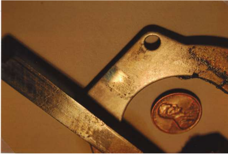
COLOR FIGURE 3.13 Polishing wear of hard steel saw components after years of service.
