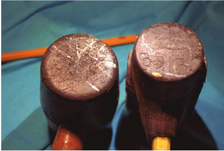
COLOR FIGURE 6.11 Impact wear on two different rubber hammers.
