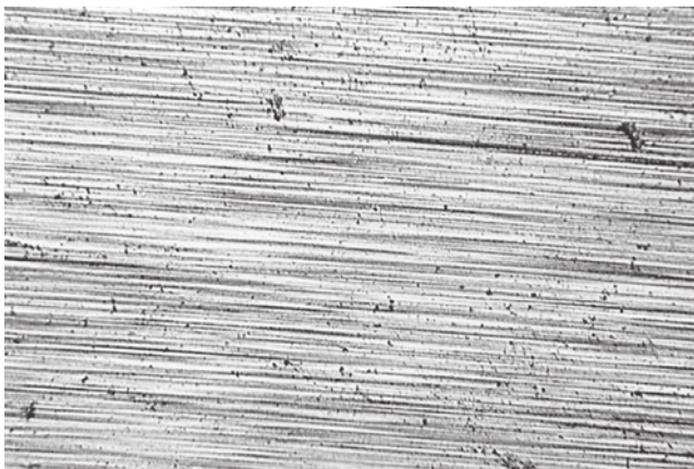
FIGURE 4.22 (a) The rubbing face of a zirconia seal. (b) The ground surface is slightly polished from the rubbing action (100 \times ).
