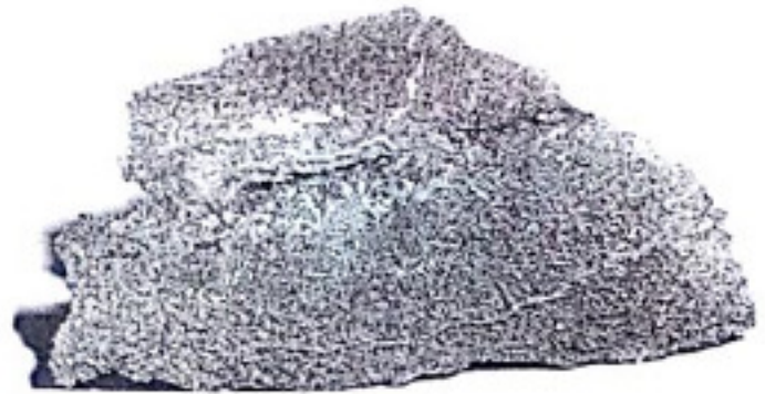
Fig. 16.6—Complete fusion of iron into the core because core was underbaked.
