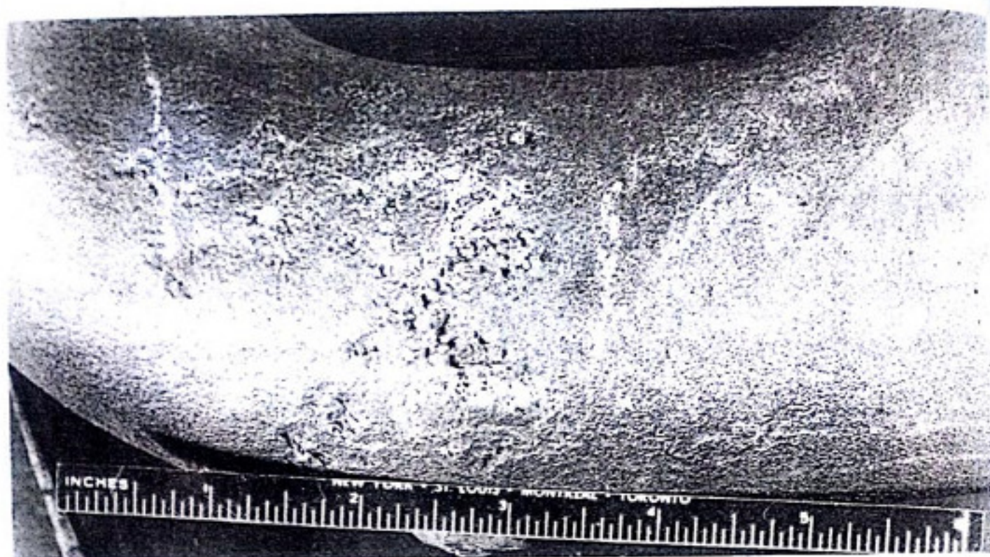
Fig. 6.11 — Metallic oxides from the ladle entered the mold until the defect was corrected by proper gating.
