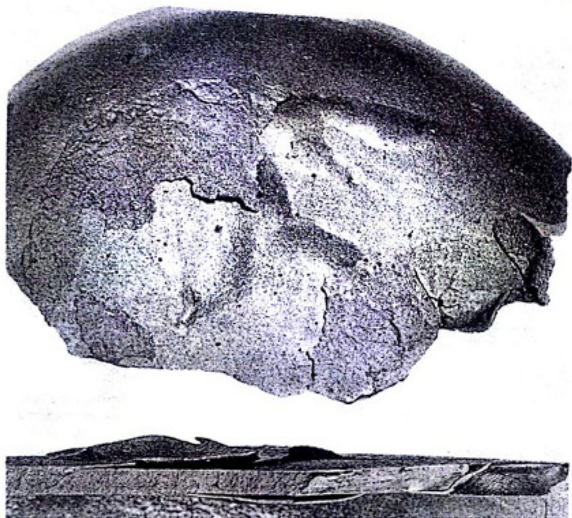
Fig. 11.14—Blister on sanitary casting caused by hard ramming and wet sand.
