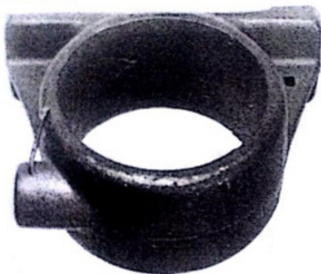
Fig. 6.3 — Poorly designed pouring basin prevented proper choke and permitted slag to enter the mold.
