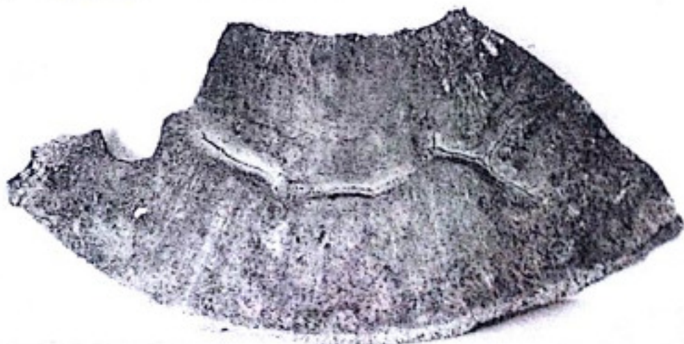
Fig. 9.6—Rat-tail caused by low clay content aggravated by high moisture in the sand.
