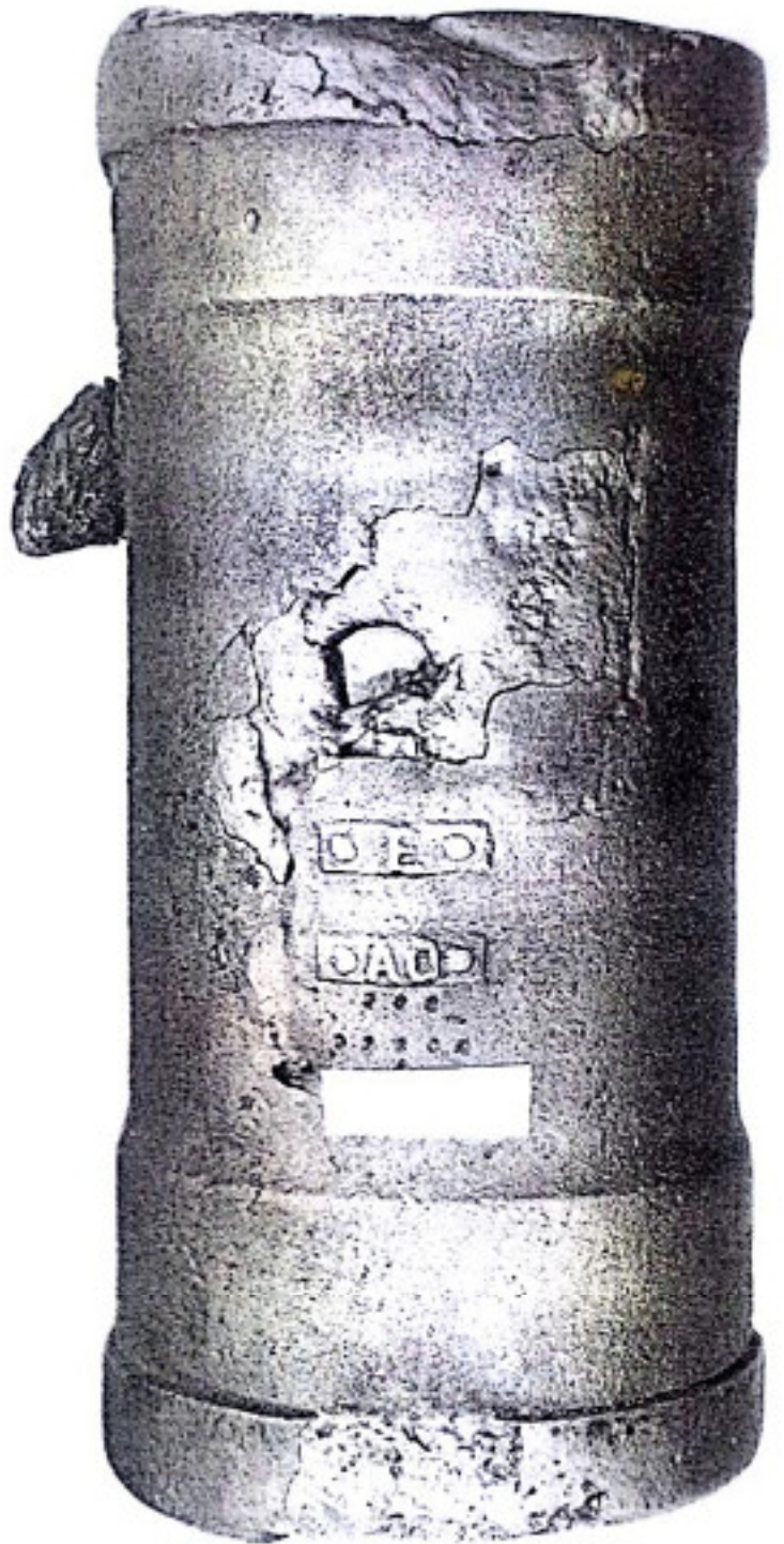
Fig. 11.6—Gas defect caused by grease from a machine fitting falling into the facing sand (foreign material).
