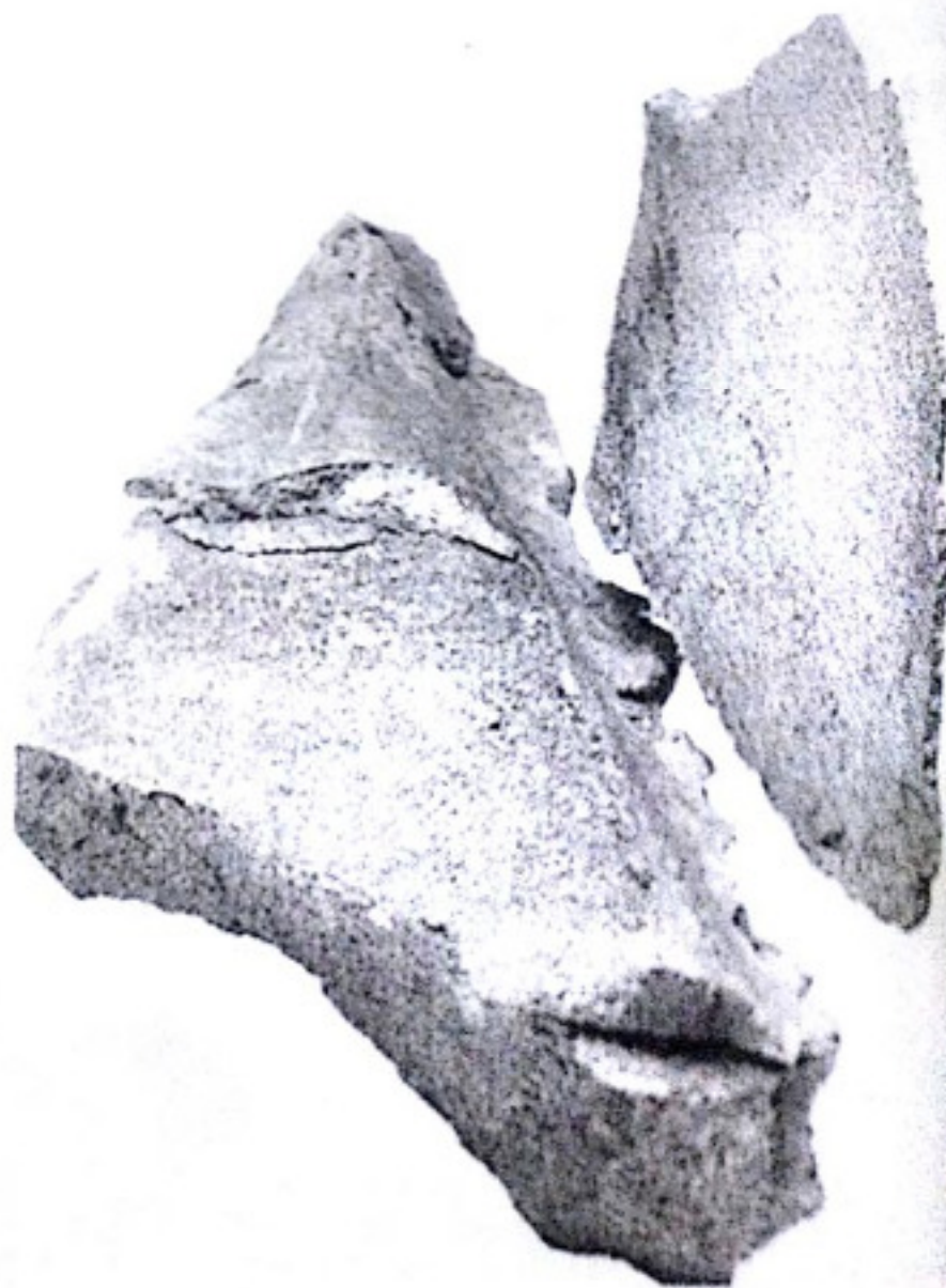
Fig. 9.10 — Blackening scabs caused by inadequate hot deformation in the sand.
