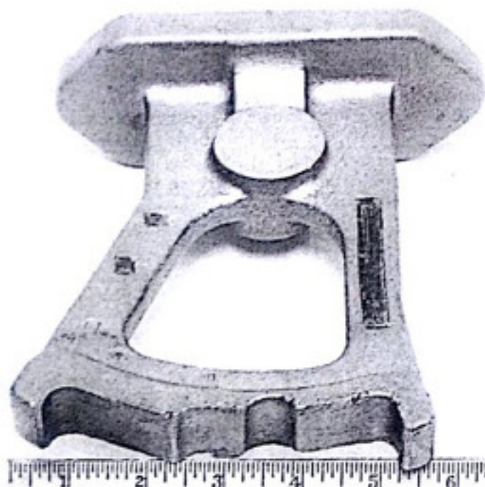
Fig. 27.2 — Cold shot from interrupted pouring.
