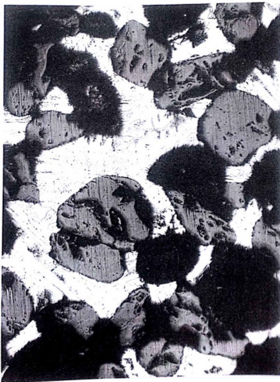
Fig. 16.3 — The photomicrograph shows the type of metal structure which is often found between the sand grains under conditions of mold porosity. \times 400 .
