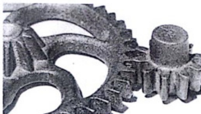
Fig. 28.9—In this small gear, a phosphorus content in excess of 0.14 per cent caused a shrinkage between the teeth.
