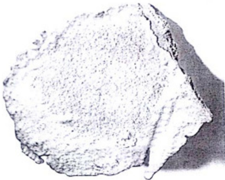
Fig. 9.11 — Expansion scab in dry sand mold after removal from the casting. This defect was caused by excessive clay wash in a gagger which was close to the casting surface.
