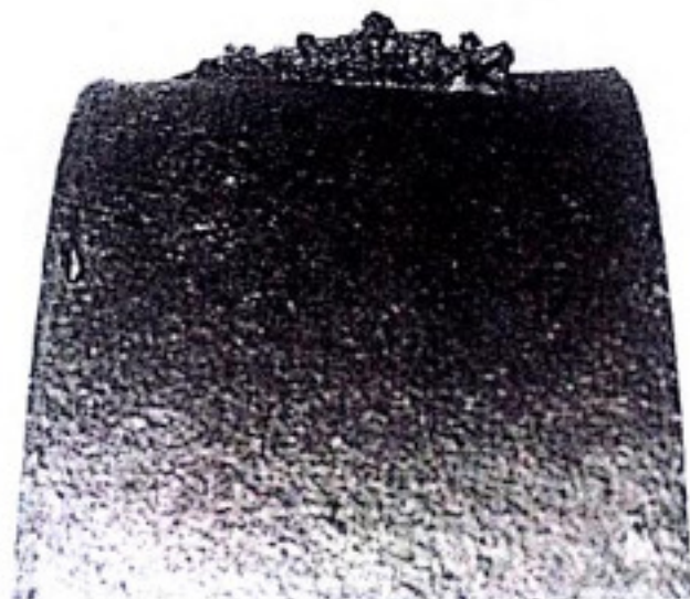
Fig. 6.12 — Two views of an inclusion caused by a rag left in the mold.
