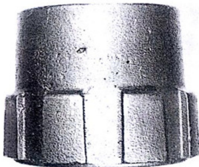
Fig. 6.6 — Loose sand left in the mold cavity by the molder causing sand inclusion on the drag face.
