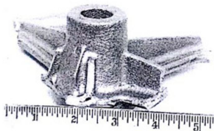
Fig. 14.3 — The casting shown was poured using a wet ladle.
