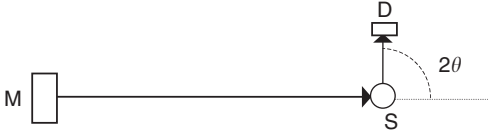
Figure 9.2 The basic components of a time-of-flight diffractometer.
