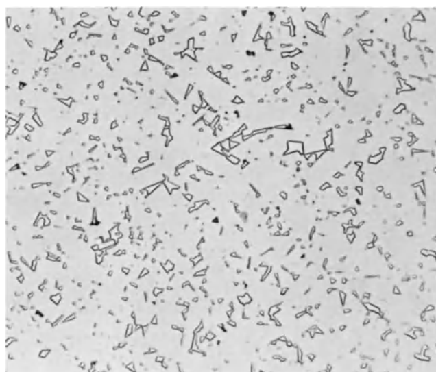
Fig. 1-3. In the as-polished condition, porosity and graphite can be observed on WC-Co samples (left). Relief polishing outlines the cobalt binder phase (right). (Both at 1000 \times .)
