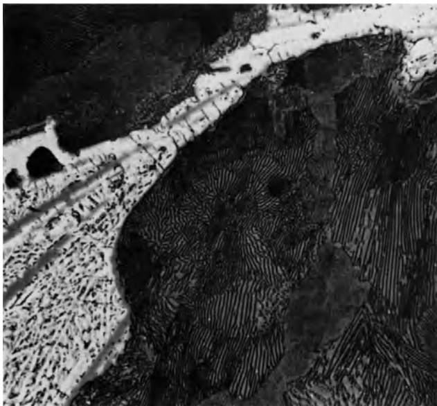
Lead Sulfide Tint Etch (etch 3h) \text{Fe}_3\text{C} pale blue
