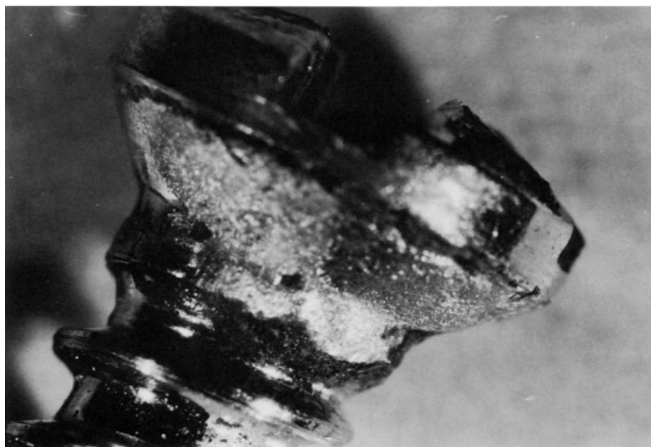
Fig. 17-3. Crevice corrosion on the head of a surgical stainless-steel screw used to fixate a bone plate to the femur to facilitate bone union.
