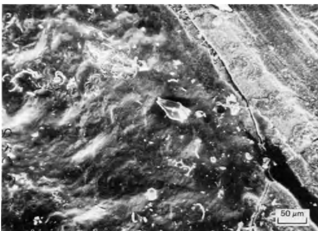
Fig. 16-6. Fretted surface of turbine blade root with a fretting fatigue failure; note fatigue crack at edge of fretted zone.
