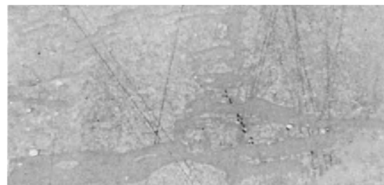
Fig. 3-12. Same microstructure area of same alloy with same preparation as in Fig. 3-11, but with a smeared surface layer as a result of improper polishing (at 500 \times ).
