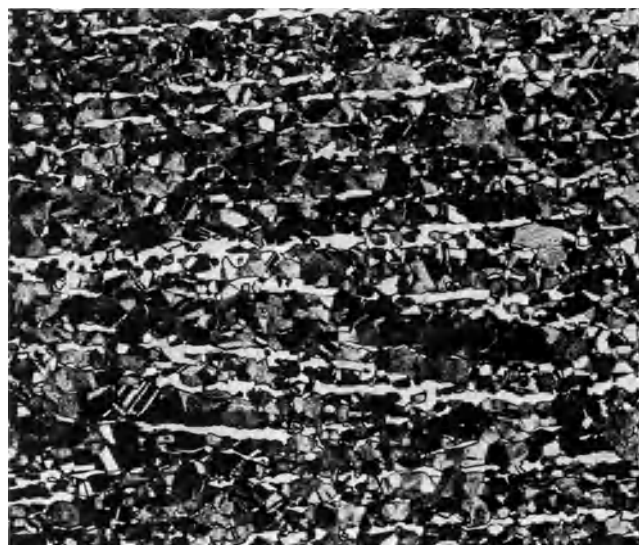
\text{NH}_4\text{OH}/\text{H}_2\text{O}_2(3\%)/\text{H}_2\text{O} (swab, etch 3b)
