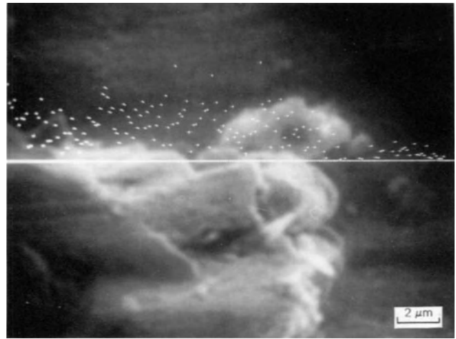
Fig. 16-12. Scanning Auger micrograph of bronze-bearing surface showing iron transfer; dots show iron concentration to a depth of 5 nm.
