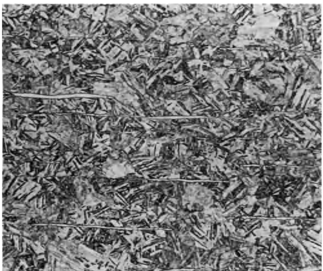
Fig. 1-14. Delta ferrite stringers in 17-4 PH stainless steel revealed (top) with 20-percent aqueous NaOH (20 V dc for 21 sec) and (bottom) by matrix etching with Fry's reagent. [100 \times (left) and 500 \times (right).]
