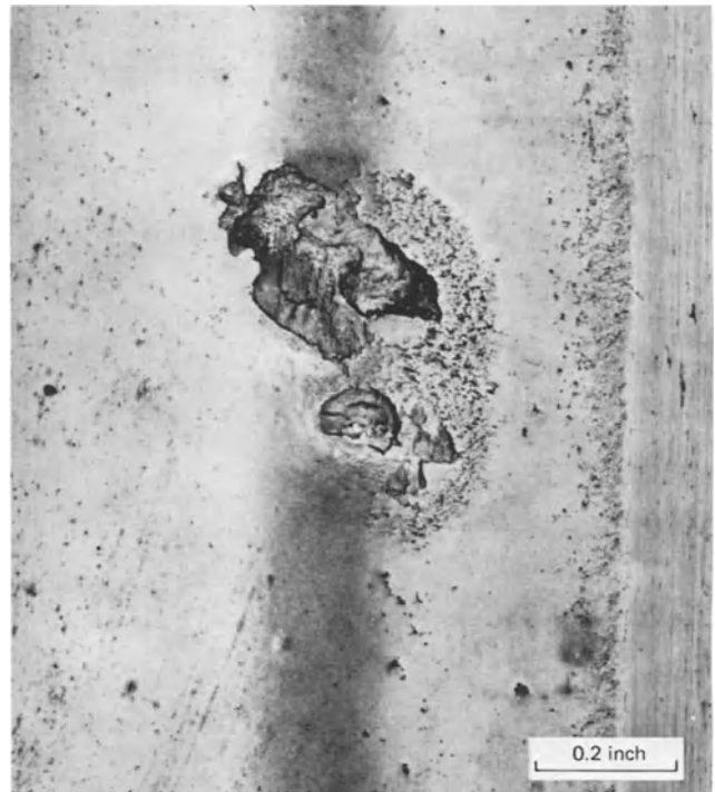
Fig. 16-10. Example of rolling-contact fatigue spalls: Micrograph of a ball bearing race (5 \times ).
