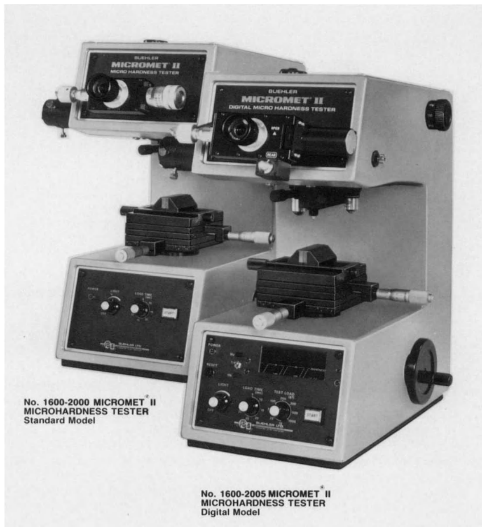
Fig. 9-9. Two compact digital and manual reading machines (Courtesy Buehler Ltd).
