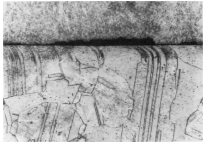
Fig. 16-23. Metallographic section through wear scar showing near-surface deformation delineated by grain-boundary bending (section was cut parallel to direction of sliding contact).
