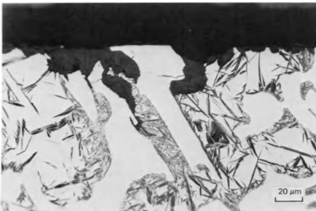
Fig. 16-22. Example of corrosive wear.
