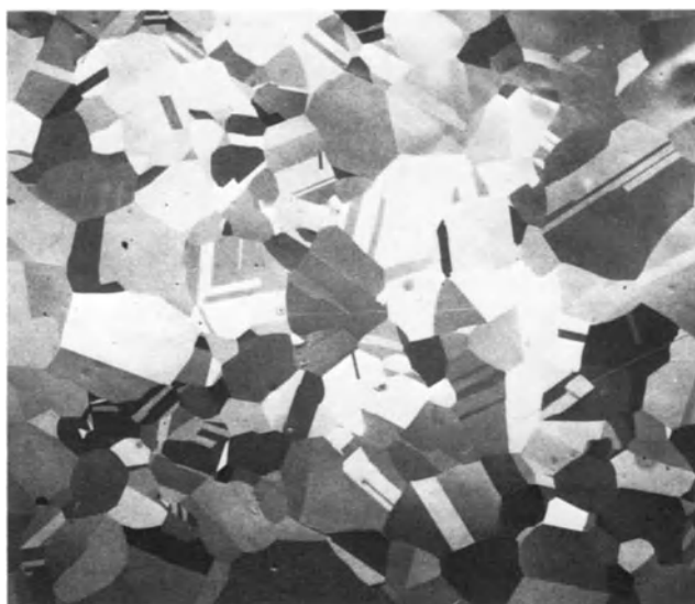
Fig. 10-6. Two examples of grain-orientation contrast with electropolished, unetched, single-phase 200 nickel using a quad-diode, solid-state backscatter detector at 30 keV (left) and the Taylor backscatter electron detector attachment at 10 keV (right), both at 100 \times .
