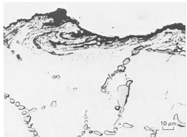
Fig. 16-28. Metallographic section of worn aluminum alloy showing mixing of surface debris in highly deformed near-surface region.
