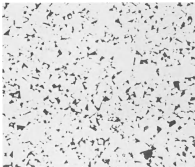
Fig. 1-18. Cobalt binder phase in WC-Co sintered-carbide cutting tool (same sample as in Fig. 1-3) revealed (left) by etching with HCl saturated with FeCl 3 (etch No. 7a) and (right) by heat tinting at 316°C for 5 min. (Both at 1000 \times .)
