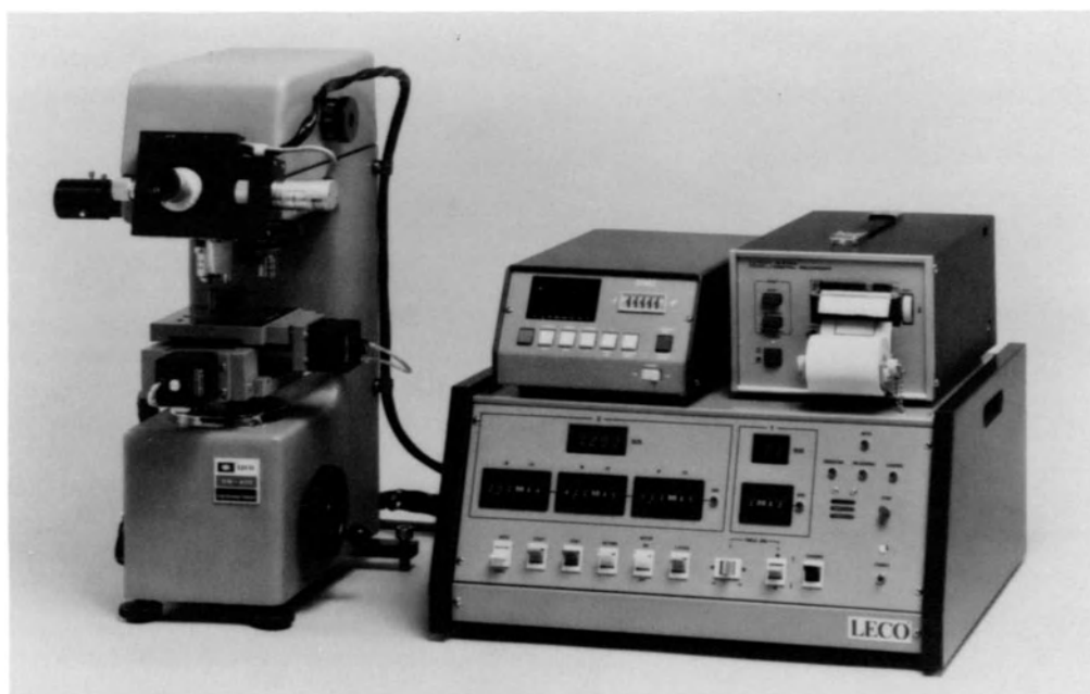
Fig. 9-8. Example of an automated programmable stage accessory for producing a prespecified test matrix of microindentations (Courtesy, Leco Corp.).
