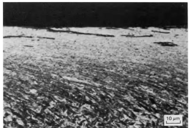
Fig. 16-24. Metallographic section from carburized chain link showing flow and subsurface cracking.
