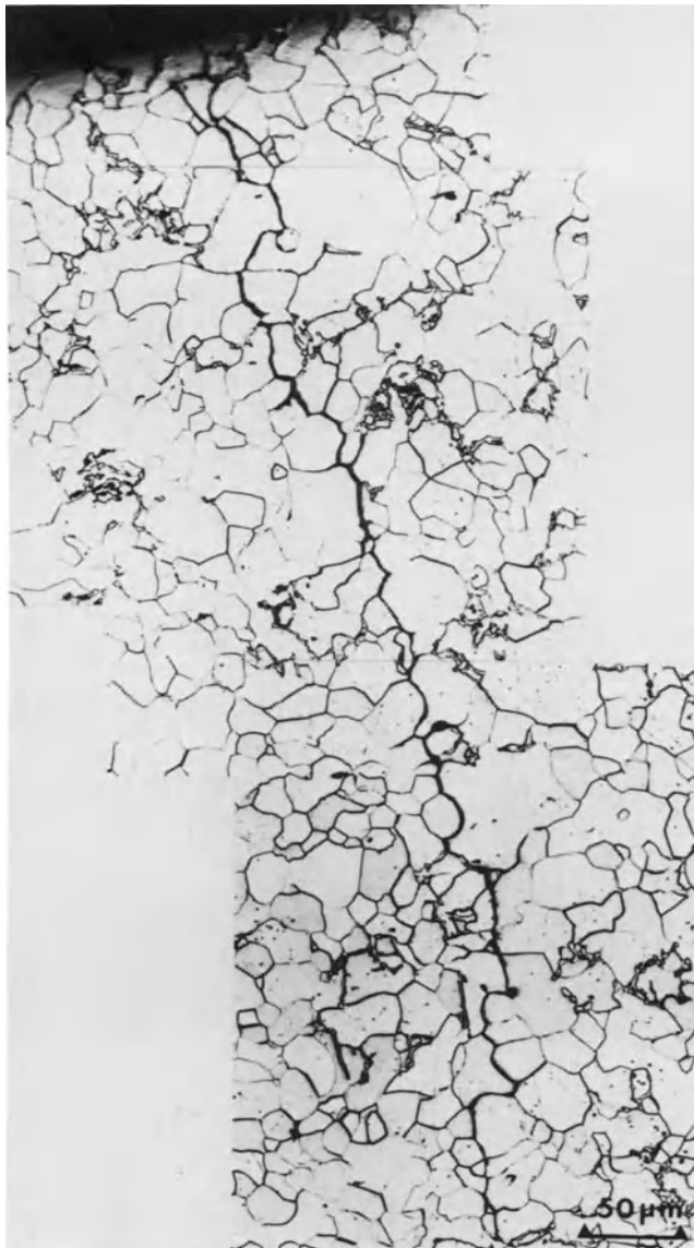
Fig. 15-20. Hydrogen-assisted cracking in a low-carbon pipeline steel; note the largely intergranular path with extensive branching (etched in nital).
