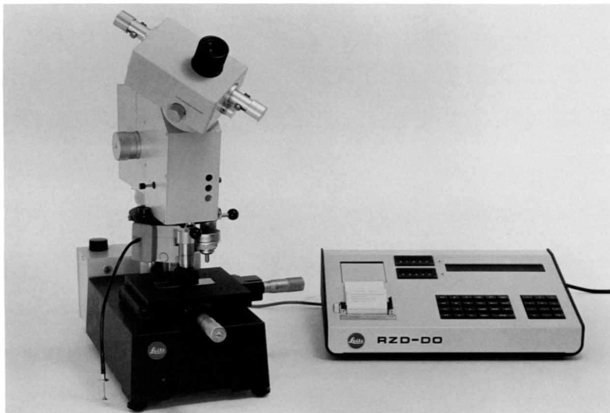
Fig. 9-7. Example of a digital measurement testing system with revolving nosepiece to allow targeting precision (Courtesy, E. Leitz).
