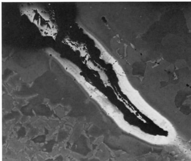
Fig. 1-13. Oxygen enrichment at a forging lap in an alloy steel revealed by Fine's alkaline chromate etch (etch No. 3i). (At 100 \times .)
