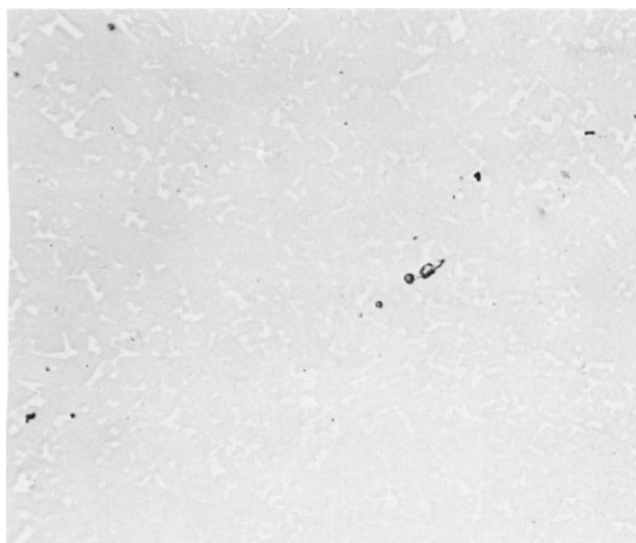
Fig. 1-3. In the as-polished condition, porosity and graphite can be observed on WC-Co samples (left). Relief polishing outlines the cobalt binder phase (right). (Both at 1000 \times .)
