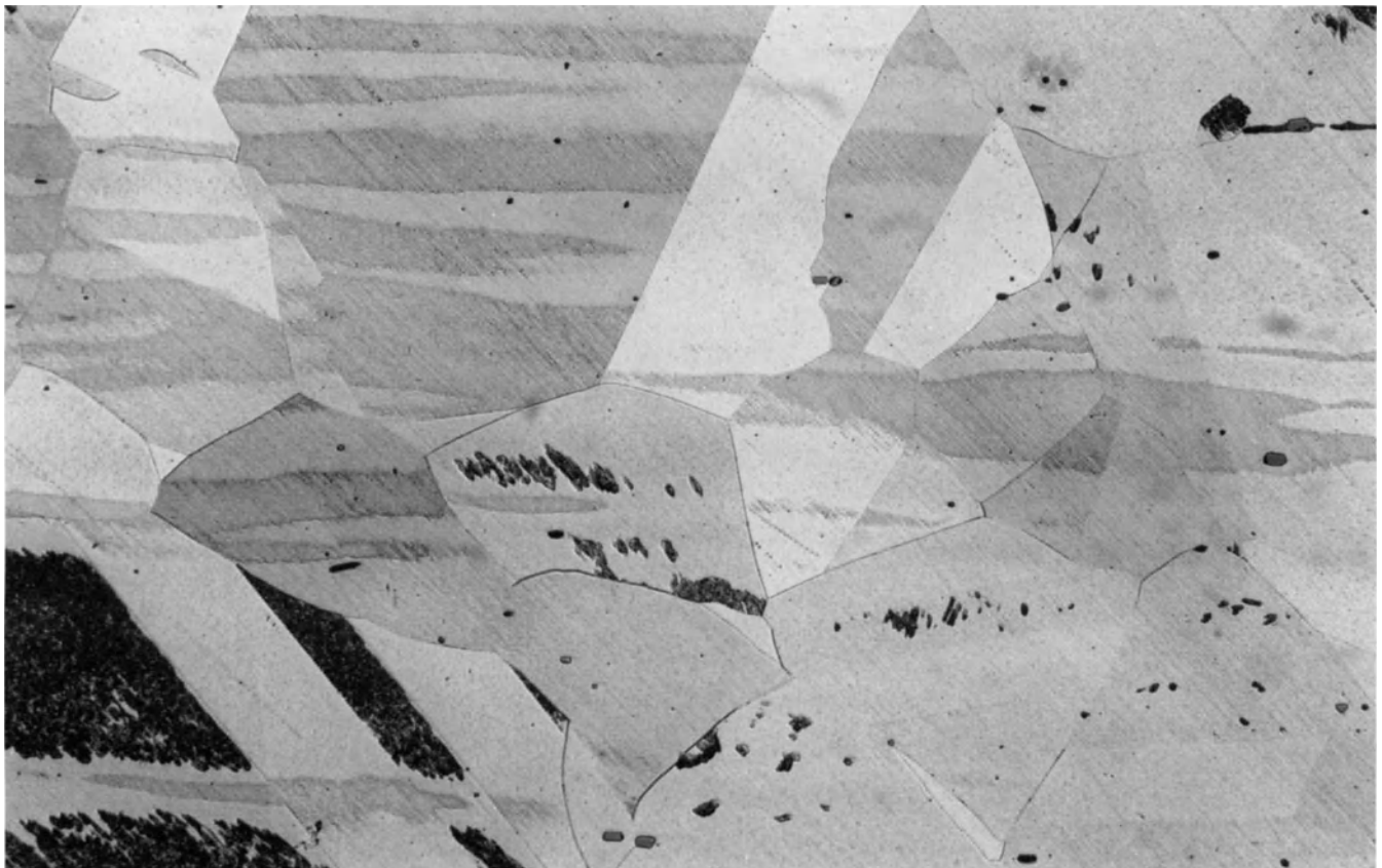
Fig. 6-5. Type 304L stainless steel: Two polishing artifacts that can occur with a low-carbon austenitic stainless steel. The dark, feathery feature is strain-induced martensite, and the mottled gray appearance of some of the grains is due to slightly disturbed metal. Etch: \text{HNO}_3 , \text{C}_2\text{H}_5\text{OH} , and sodium metabisulfite stain after Beraha. (200 \times .)
