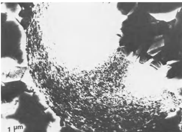
Fig. 16-26. TEM micrograph of section through wear scar showing embedding of hard wear debris in soft counter surface. (Courtesy, Tyzh-Chiang Sun, Ohio State University).
