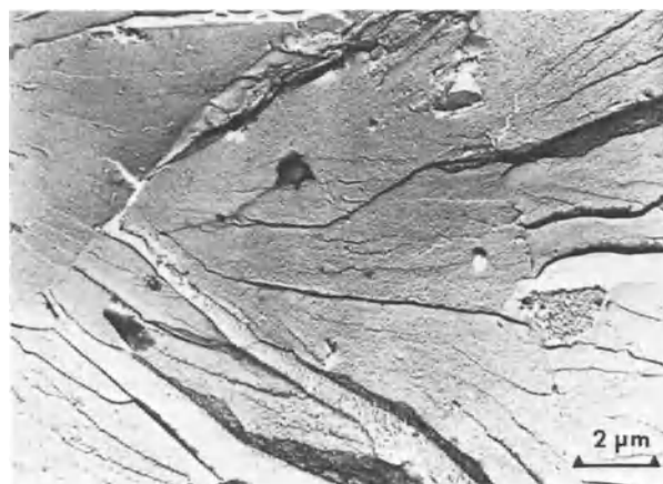
Fig. 15-2. Cleavage fracture in a mild steel bolt, showing characteristic river patterns (two-stage, plastic-carbon replica viewed in the TEM).
