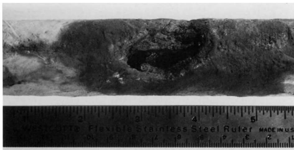
Fig. 17-1. General corrosion of a carbon-steel "Quench string" taken from a heavy oil production well: Corrosion from reservoir fluids in the well bore caused perforation of the steel tubing in several areas.
