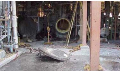
The cover plate blew off this polymer catch tank, killing three workers
