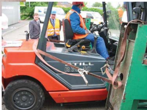
Reconstruction of the incident. The retaining strap passes behind the driver's heels
