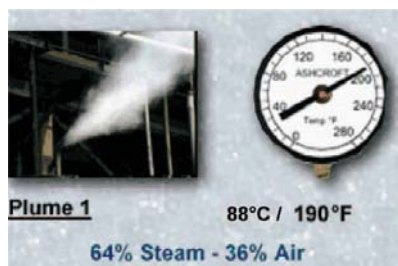
Figure 3 The gas coming out of the pipe nipple contains 64 percent steam and 36 percent air. The dial thermometer measuring the mixture temperature reads 190°F (88°C). The temperature outside was 60°F (15.5°C) when the picture was taken.
