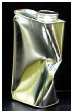
Figure 9b Result of condensation. This can was filled with steam and then closed. The steam condensed, and the resulting vacuum caused the damage shown.
