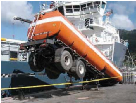
Figure 46 Care must be taken when unloading compartmentalized tank wagons!
