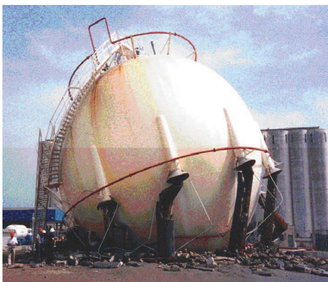
Figure 8b This sphere collapsed during an hydraulic test because legs were corroded behind fireproofing concrete. An inspector was killed.
