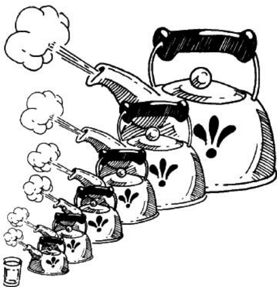
Figure 1 At 212°F (100°C) and atmospheric pressure, water expands about 1,600 times!
