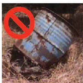
Wrong way to dispose of spent catalyst
