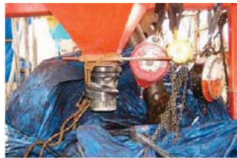
Loading hopper valve
