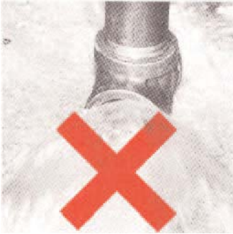
Figure 14 A tee on the end of a loading spout should not be used because it produces splash and spray which add to the generation of static electricity.
