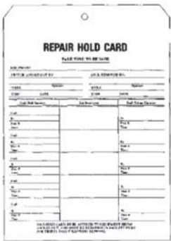
Figure 70 Typical 'Repair Hold Card'.
