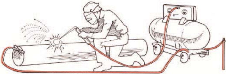
Figure 31 The ground return cable for welding machines must be attached to the object on which welding is being done.
