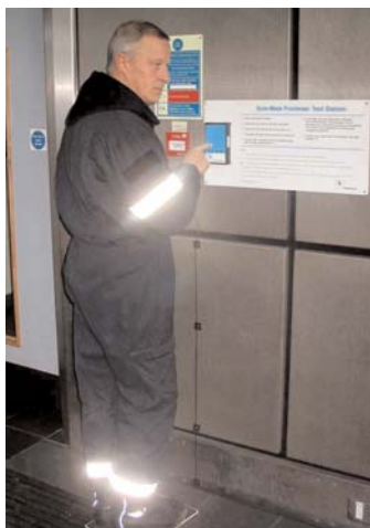
Figure 21b Refinery operator testing his shoes at the beginning of his shift for an anti-static conductivity between 10 and 50 ohms.
