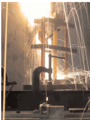
Figure 22 Picture of a floating roof to shell shunt test (submitted to a 830 A current to simulate lightning) showing the sparks generation (note that wax and rust deposits increase sparking).
