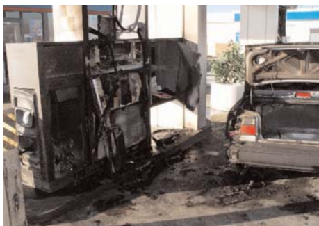
Pumps and car damaged after a static electricity discharge ignited gasoline vapours in a US service station.
