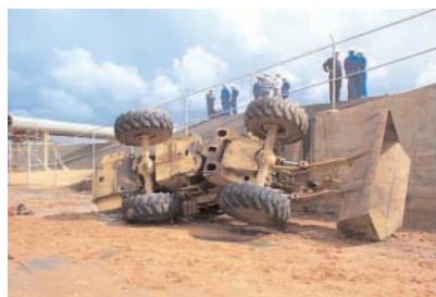
(Top left) This is the pig trap after the incident. (Right) The large front end loader was completely flipped over by the ejected foam pig.
