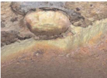
(Left) Polymer plugging the polymer catch tank vent nozzle. (Right) Vent line obstructed by solid polymer.
