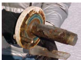
Outlet branch with plug of ice.
