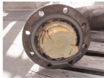
(Left) Polymer plugging the polymer catch tank vent nozzle. (Right) Vent line obstructed by solid polymer.
