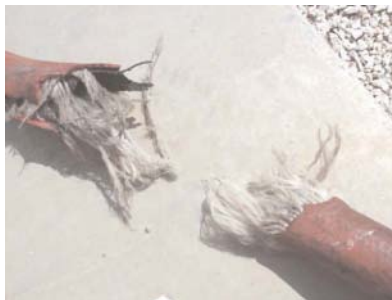
Ruptured nitrogen hose due to high backpressure.
