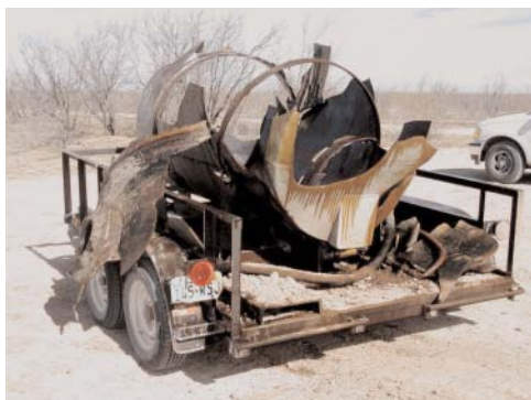
The ruptured blowdown tank.
