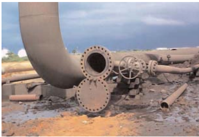
(Top left) This is the pig trap after the incident. (Right) The large front end loader was completely flipped over by the ejected foam pig.
