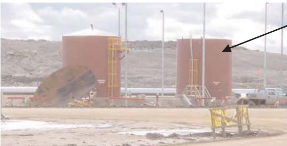
Tank after roof blew off.
