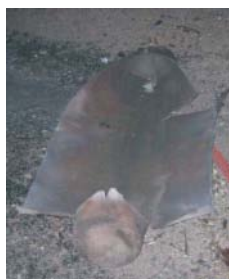
This gas bottle was involved in a spill fire and exploded.
