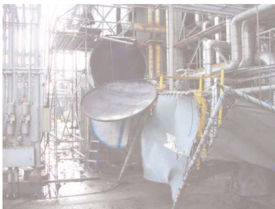
The insulated flat-head horizontal cylinder failed due to overpressure.
