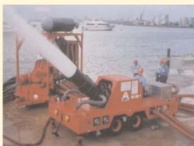
Example of a non-aspirated monitor with large mobile pump
