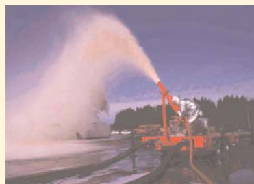
Example of a large aspirated monitor
