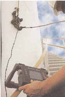
Crawler that can climb a tank and measure the tank shell wall thickness.
