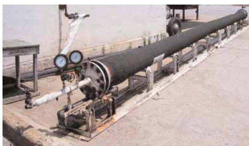
Hydraulic test apparatus for proving integrity of hoses at periodic intervals
