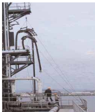
Well supported hose during lifting
