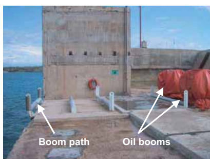
Some clean-up tools for oil spills
