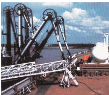
Safe access from shore to ship for terminal representative and ship's crew
