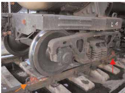
Chocks located beneath wheels of rail truck to prevent movement
