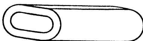
Fig. 1. Flattening test for tubes in the M condition
