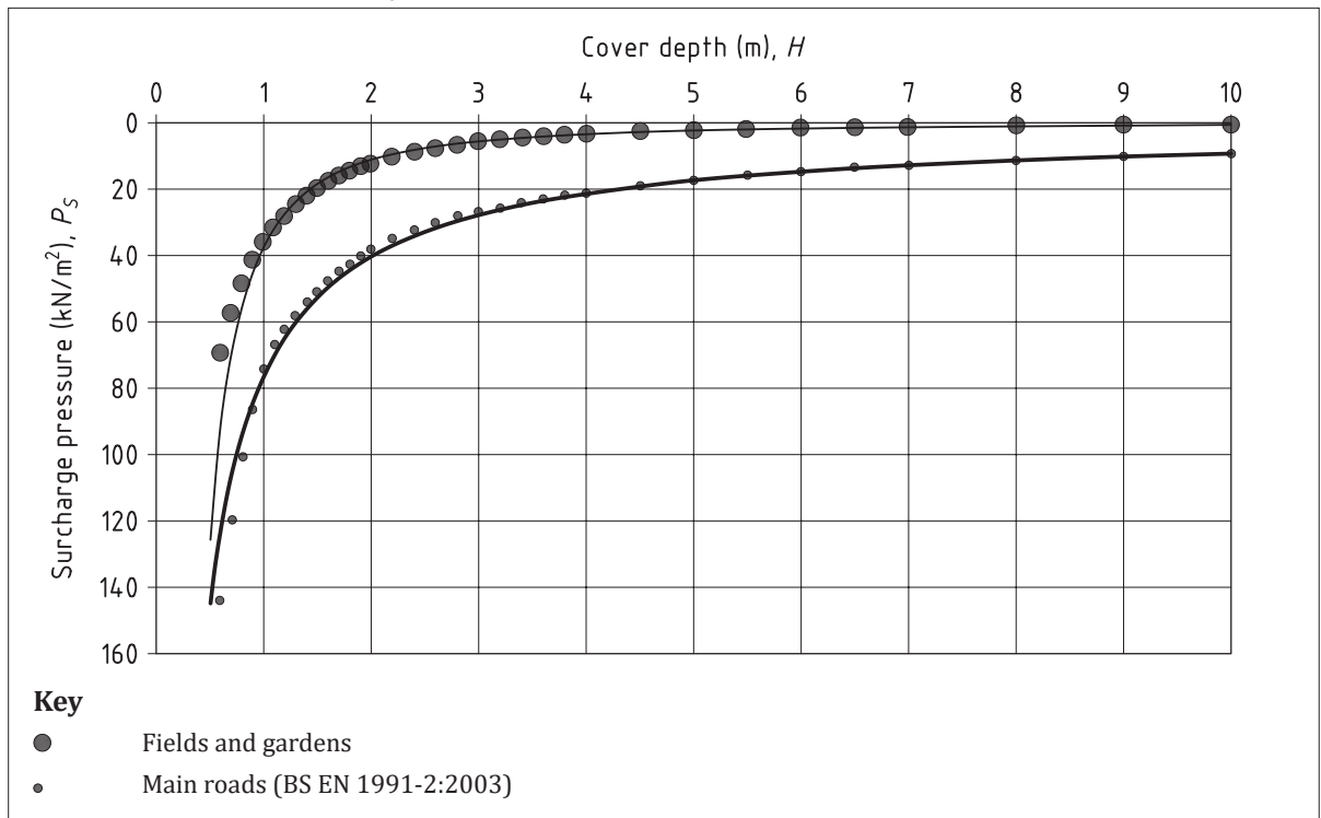
Figure 9 — Surcharge pressure ( \text{kN/m}^2 ), P_s , due to vehicle wheels
