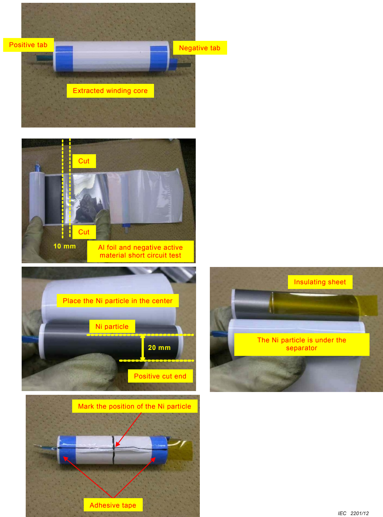
Figure A.5 – Disassembly of cylindrical cell
